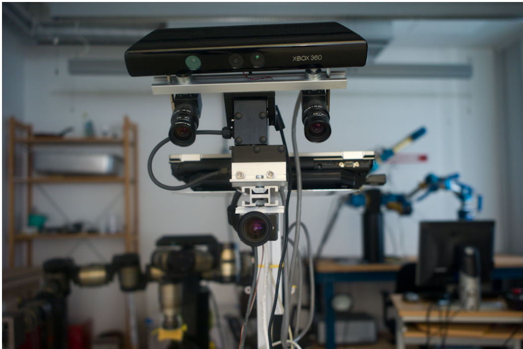
Figure 1.2: Microsoft Kinect mounted on a mobile robot platform at CVAP (KTH)
