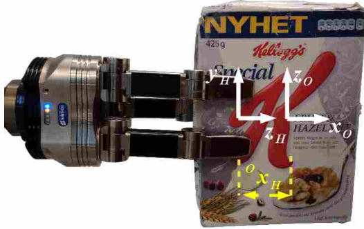
Fig. 5 : Grasp preshape used for training on the maximum static friction forces and torques, with the corresponding reference frames of the hand and the object used for training.
