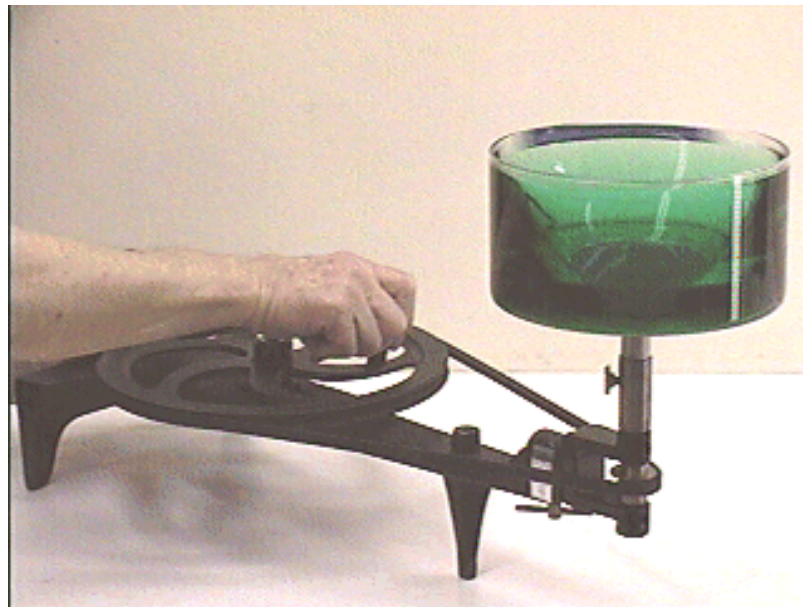
Figure 19.1: Newton: Look at the curved water surface of the spinning bucket of water caused by inertial forces. Do you think that it is the bucket of water which is spinning, or do you (like Mach and Einstein) believe that (possibly) the Universe is spinning around the bucket subjecting the water to some mysterious gravitational pull?
