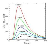
Figure 3: Radiation energy vs wave length/frequency at different temperatures of a radiating blackbody, per unit frequency. Observe that the cutoff shifts to higher frequency with higher temperature according to Wien's Displacement Law.
