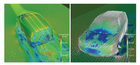
*Figure 8*: Velocity of turbulent G2 flow with slip around a car with courtesy of geometry Volvo Cars and computations by Murtazo Nasarov.
