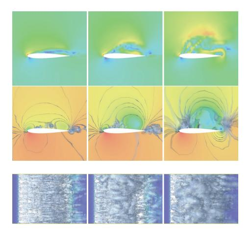
*Figure 6*: G2 computation of velocity magnitude (upper), pressure (middle), and non-transversal vorticity (lower), for angles of attack 20, 22, and  $24^{\circ}$  (from left to right).
