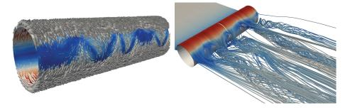
*Figure 9*: Turbulent separation by surface vorticity forming counter-rotating low-pressure rolls in flow around a circular cylinder, illustrating separation at the trailing edge of a wing [23].
