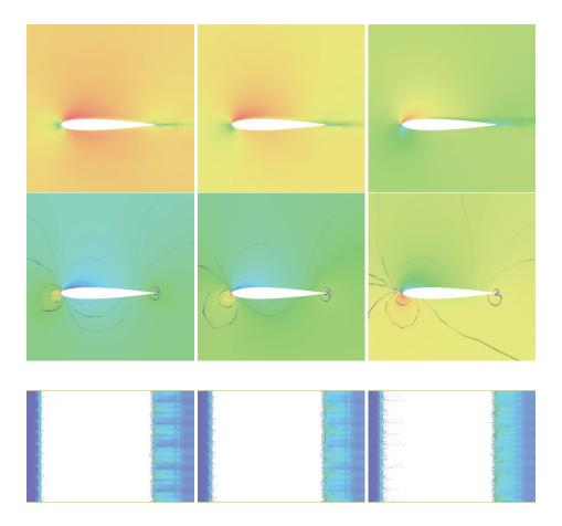
*Figure 4*: G2 computation of velocity magnitude (upper), pressure (middle), and non-transversal vorticity (lower), for angles of attack 2, 4, and  $8^{\circ}$  (from left to right). Notice in particular the rolls of streamwise vorticity at separation.
