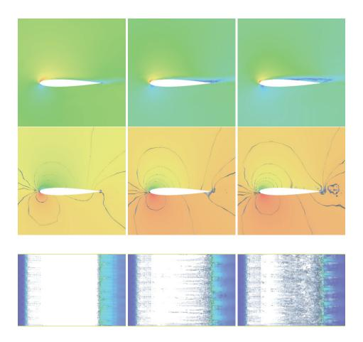
*Figure 5*: G2 computation of velocity magnitude (upper), pressure (middle), and topview of non-transversal vorticity (lower), for angles of attack 10, 14, and  $18^{\circ}$  (from left to right). Notice in particular the rolls of streamwise vorticity at separation.
