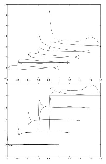
*Figure 7*: G2 computation of normalized local lift force (upper) and drag force (lower) contributions acting along the lower and upper parts of the wing, for angles of attack 0, 2, 4, 10 and  $18^{\circ}$ , each curve translated 0.2 to the right and 1.0 up, with the zero force level indicated for each curve.
