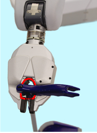
Fig. 12. A PR2 gripper caging a scoop by an approximate caging loop
