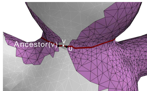
Fig. 15. Illustration of Alg.3. Currently explored vertices and edges are depicted in black; faces whose edges and vertices are black, are depicted in purple and a resulting caging loop is shown in red.
