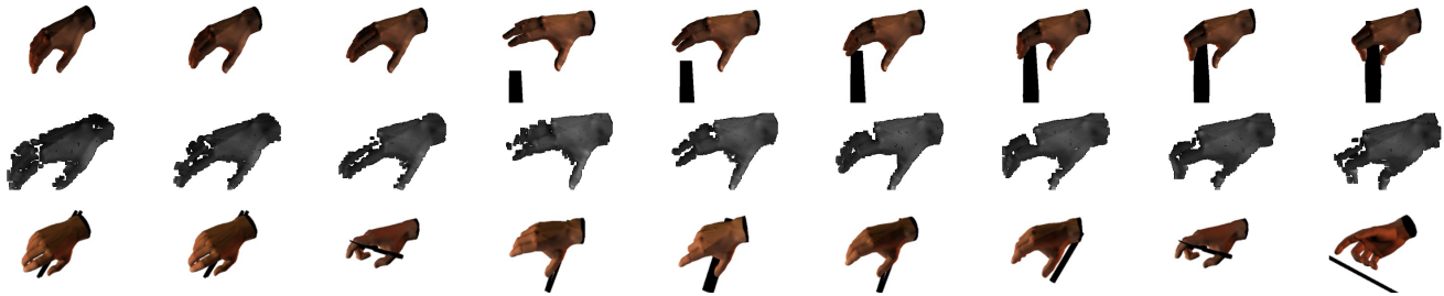
Fig. 6. Synthetic sequence 1. Top: original synthetic image. Middle: segmentation image with \alpha = 0.5\% . Bottom: estimated pose. (The objects in the database are colored black for visibility here, but do not contribute to the HOGs.) Video at www.csc.kth.se/~jrgn/VideosICRA2010/synthetic1.mp4
