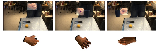
Fig. 14. Real sequence 5 (male subject 1) with fast non-linear motion. Top: image with skin segmentation window highlighted. Bottom: estimated pose. Video at www.csc.kth.se/~jrjn/VideosICRA2010/real5.mp4
