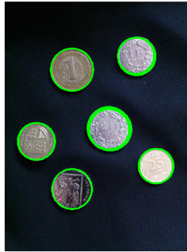
Figure 2: Circles detected with Hough transform.
