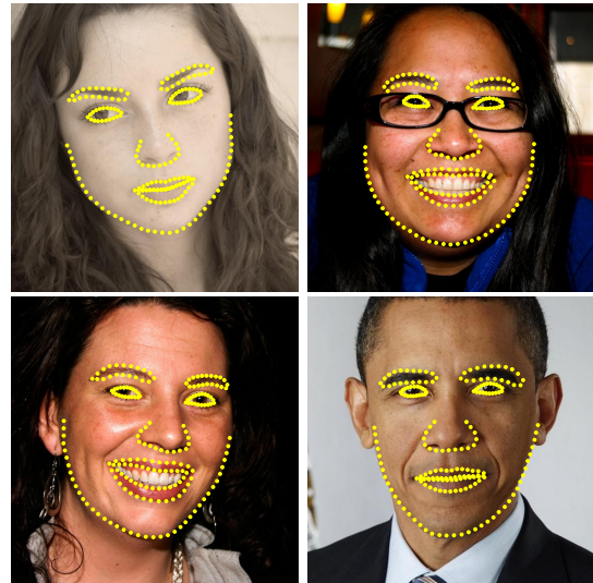
Figure 1. Selected results on the HELEN dataset. An ensemble of randomized regression trees is used to detect 194 landmarks on face from a single image in a millisecond.
