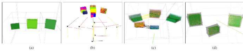
Figure 2.9: Ego-motion Estimation observing a Dynamic Scene. a) 3D blob map at the first registration is displayed, b) shows the pose frames that were reached by the robot and the sequence of static registrations enumerated by color: 1-green, 2-yellow, 3-orange, 4-blue, 5-red, 6-light blue 7-pink, the blob at the right was not moved, hence, all the registrations (colors) are overlapped on it; c) motion detection of two objects between poses 4-blue and 5-red are detected in the map, the scene is observed from above, d) shows the updated map at the end of the sequence.
