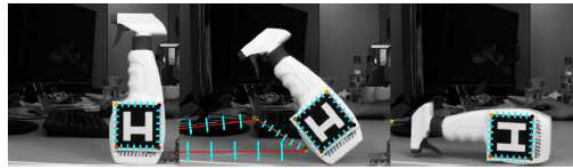
Figure 2.6: Active striking of an object to perform system identification: mass center and mass distribution from observation
