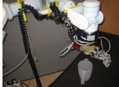
Fig. 1. PA-10 7 d.o.f with Barrett Hand and a JR3 force/torque and acceleration sensor. The hand has Weiss Robotics pressure sensors on its fingertips.
