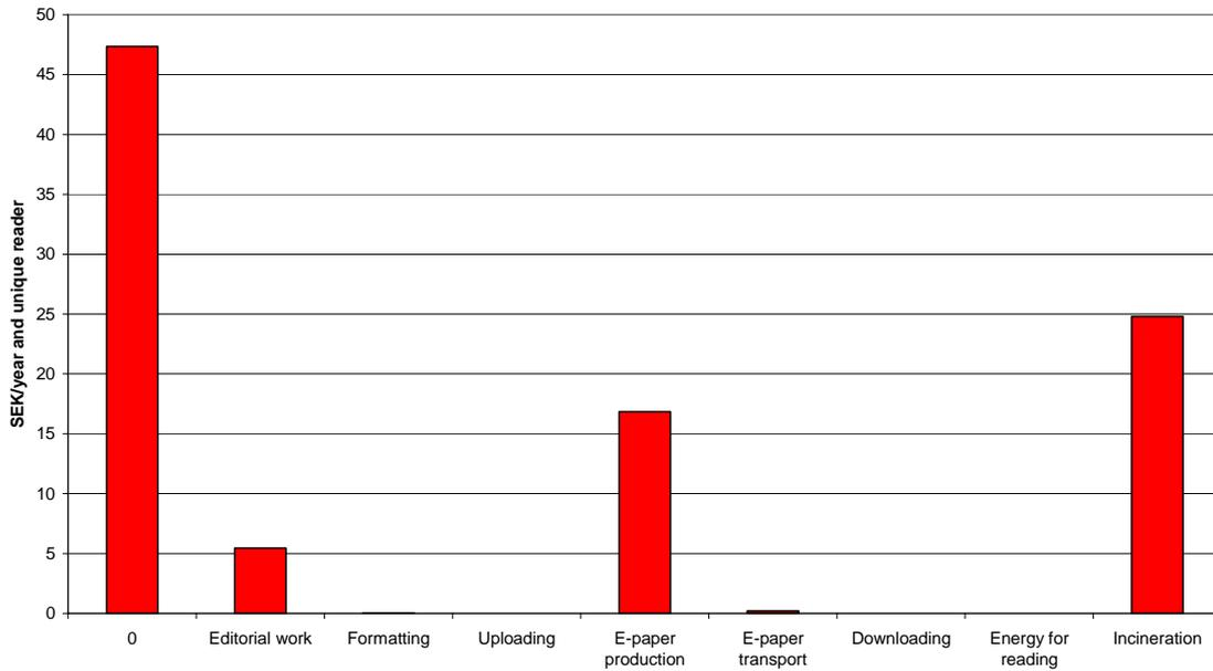
Figure 48. The total weighted values for different parts of the tablet e-paper newspaper life cycle in the Swedish scenario using the Ecotax 02 min weighting method.
