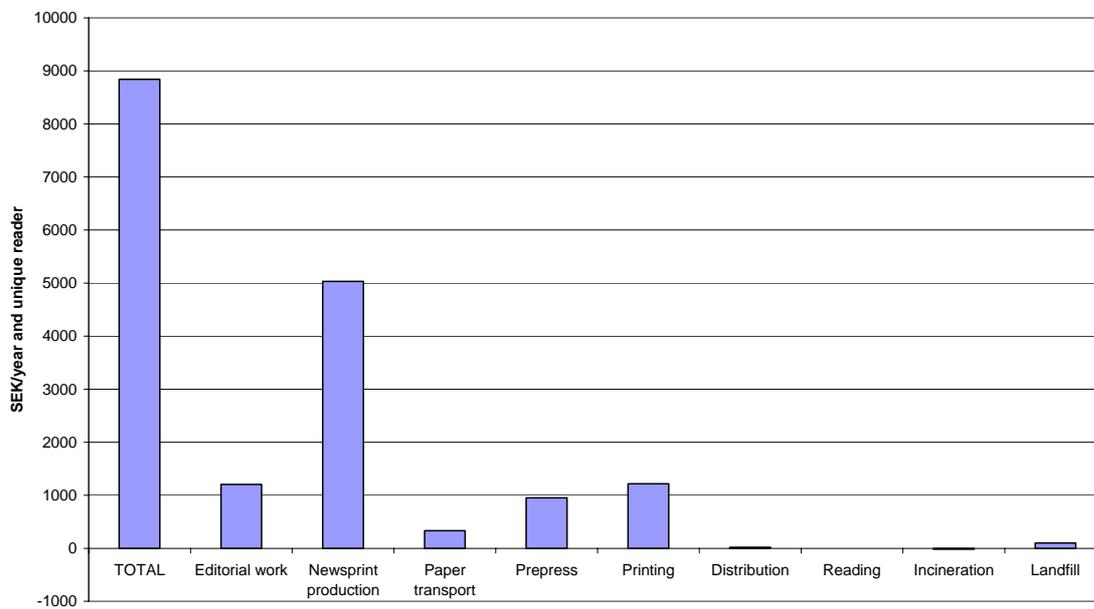
Figure 14. The total weighted values for different parts of the printed newspaper life cycle in the European scenario, using the Ecotax 02 max weighting method.
