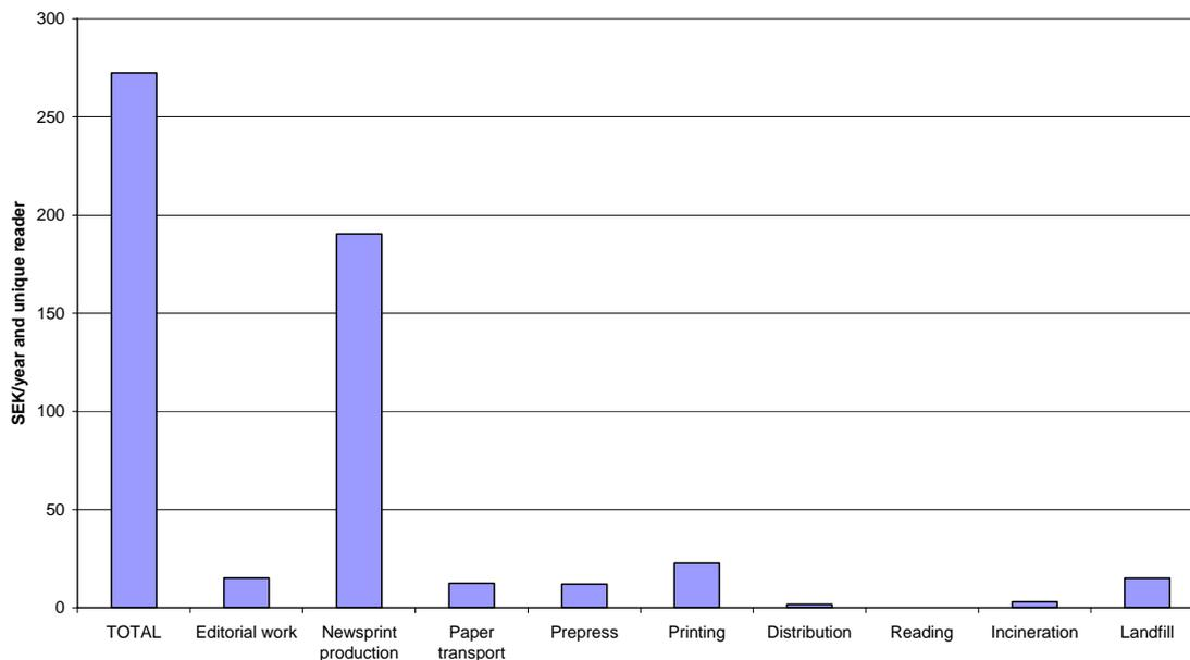
Figure 13. The total weighted values for different parts of the printed newspaper life cycle in the European scenario, using the Ecotax 02 min weighting method.
