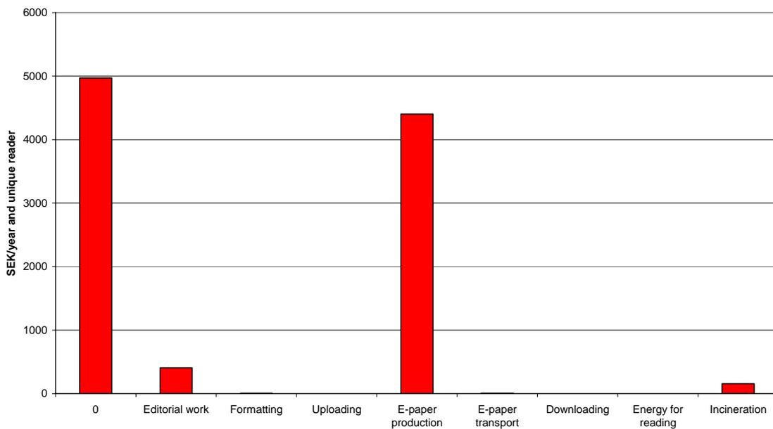
Figure 49. The total weighted values for different parts of the tablet e-paper newspaper life cycle in the Swedish scenario using the Ecotax 02 max weighting method.
