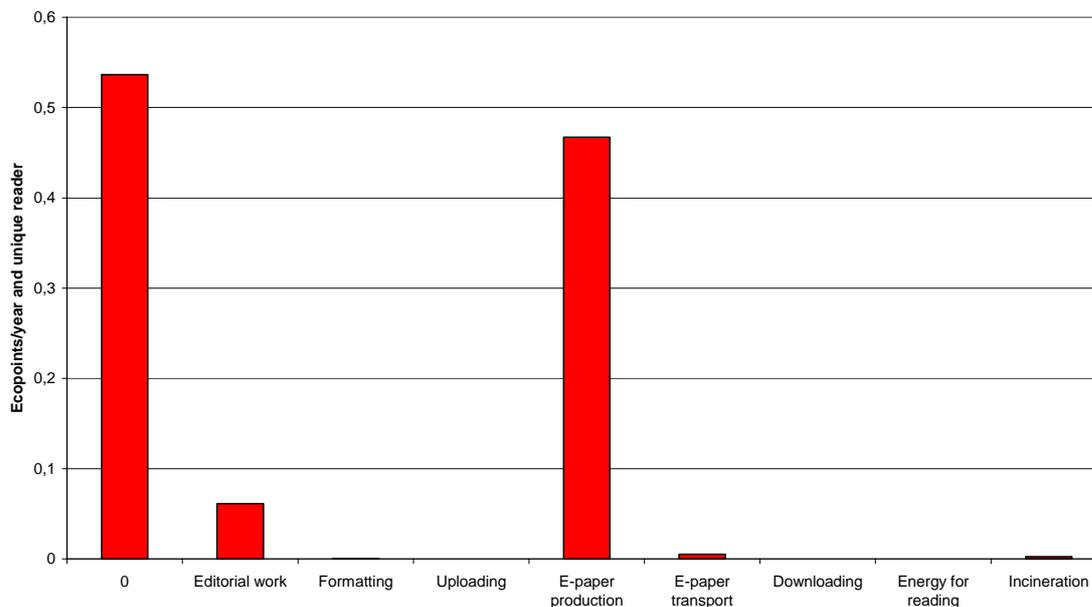
Figure 50. The total weighted values for different parts of the tablet e-paper newspaper life cycle in the Swedish scenario using the Ecoindicator 99 (HA) weighting method.
