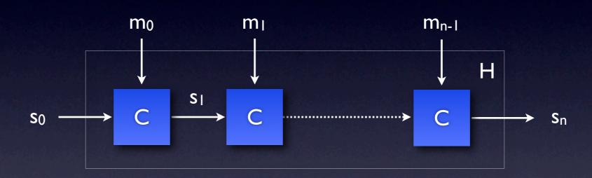
The Merkle-Damgård scheme builds a collision resistant hash function H from a collision resistant compression function C.
