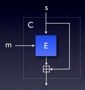
The Davies-Meyer scheme builds a compression function  $\mathcal C$  from an encryption function  $\mathcal E$ .
