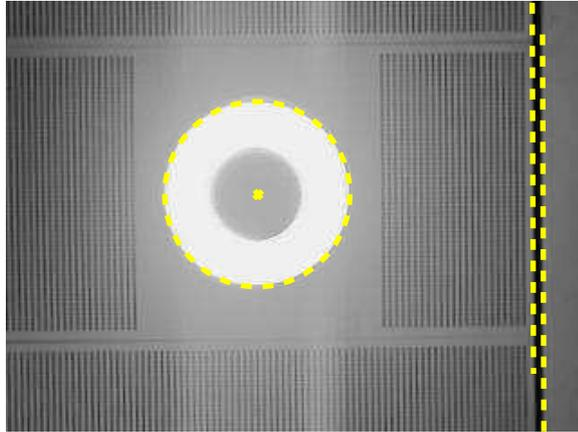
Figure 5.5: Example image with two line features and a lamp feature detected.
