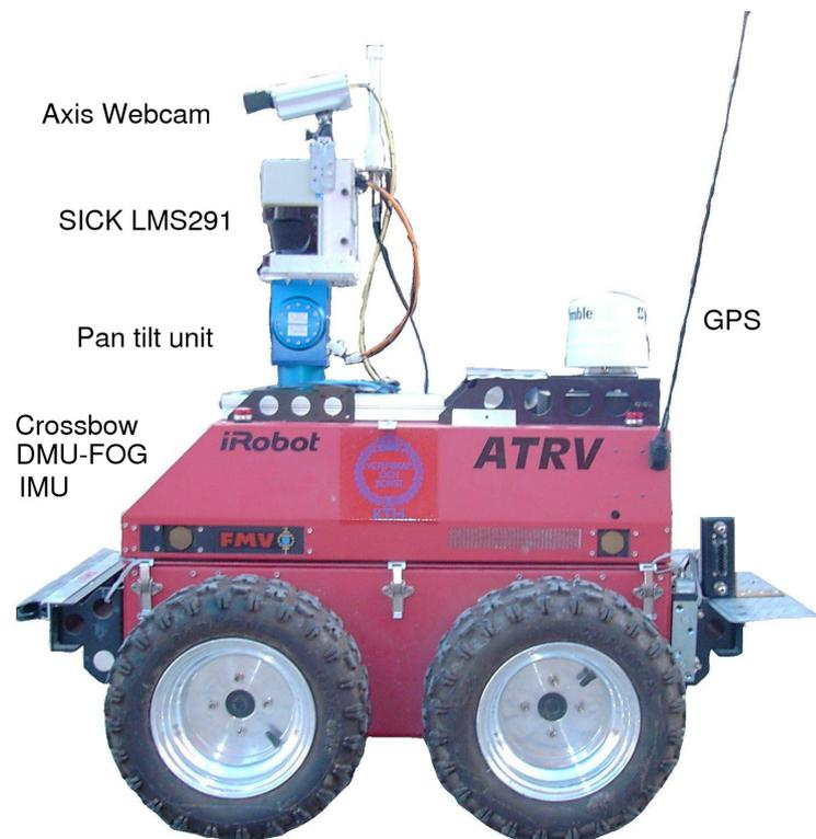
Figure B.2: Here is our ATRV Robot, Pluto.
