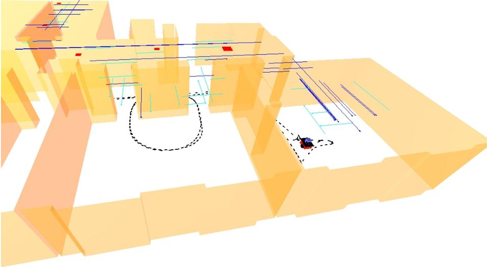
Figure 5.8: The same map from another viewing angle. One can see that the features are indeed 3D. The ceiling height is higher in the rooms than in the hallway.
