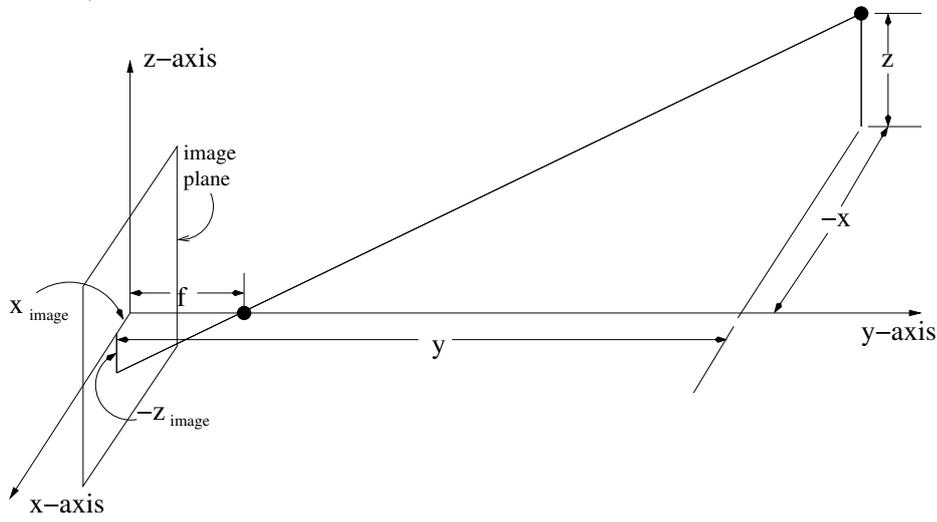
Figure 4.4: The camera is pointing in the y direction and the center point of the image plane is at the origin.
