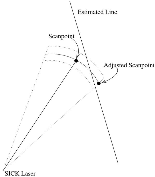
Figure 4.2: The SICK laser range point angle is adjusted to agree with the assumptions of a smooth line and a finite constant beam width. In the situation illustrated the right side of the beam will be the first to be reflected back to the scanner.
