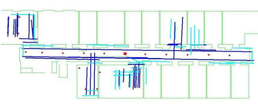
Figure 5.9: This shows a larger, (13 m x 39 m), EKF map made using vision features on the ceiling with the pioneer robot. The building walls are shown for reference only and were not part of the SLAM estimate. The darker lines are the full 3D horizontal ceiling lines while the lighter (blue) ceiling lines are one dimensional (orientation only). The squares show the locations of ceiling lamps.
