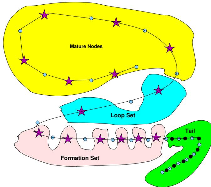
Figure 6.6: This figure illustrates the four sections of the graph. No feature nodes are shown for clarity. The tail is the newest section of the graph where no star nodes have yet been formed. The formation set is where the stars are being built up until they become too large to grow any more. They are then moved to the loop set which is matched to the mature nodes to find possible loops in the graph. After searching for loops the stars from the loop set are moved to the mature nodes.
