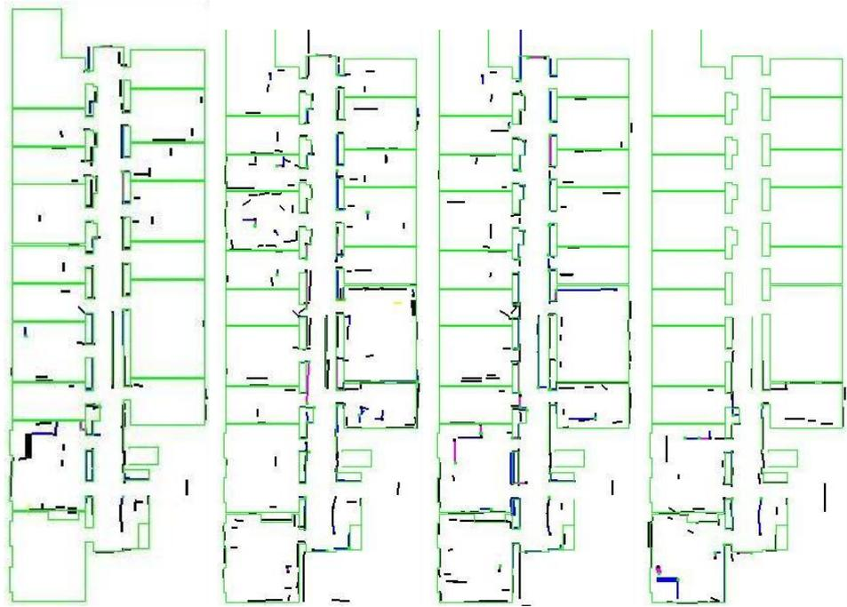
Figure 5.2: Four EKF maps made by from left to right a PeopleBot, Pioneer, PowerBot and a custom built robot. The number of walls in the maps were 120, 232, 218 and 86 respectively. The lighter (green) lines represent the hand made map while the darker (black) lines are the SLAM map. The size of this building is 13 by 39 meters.
