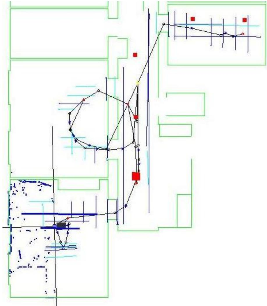
Figure 6.7: Here is the map made using the star nodes and vision features indoors. The size of the mapped area is about 13 by 15 meters. The robot path starts and ends in the room at the lower left. The raw laser scan data is displayed as a check on the final localization accuracy. By comparing it to the hand made map shown by the lighter (green) lines, one can assert that the final location was accurate to a less than 5 cm.
