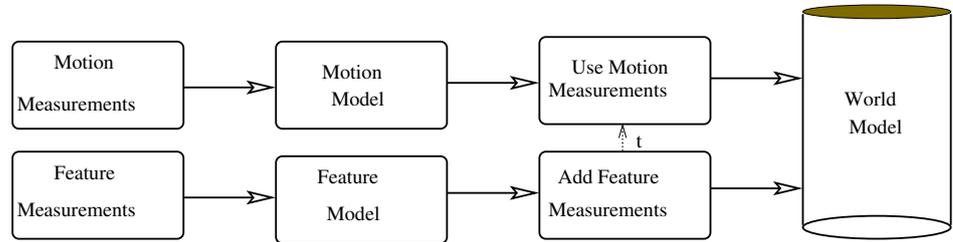
Figure 2.1: The SLAM estimation problem is split between a part that uses the motion measurements to predict the robot motion up the time of the feature measurements and a part that uses the feature measurements to update the world model.
