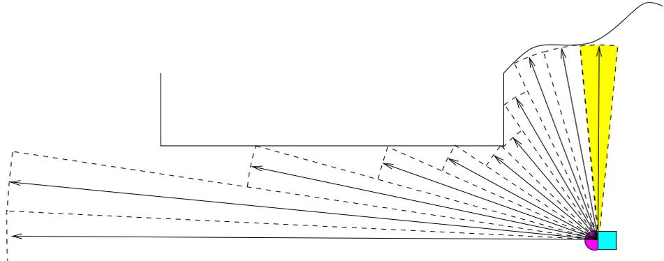
Figure 4.1: An illustration of the SICK laser scanner showing half of a complete scan, one quadrant. The beam width has been exaggerated for illustration and the number of range measurements per scan reduced.
