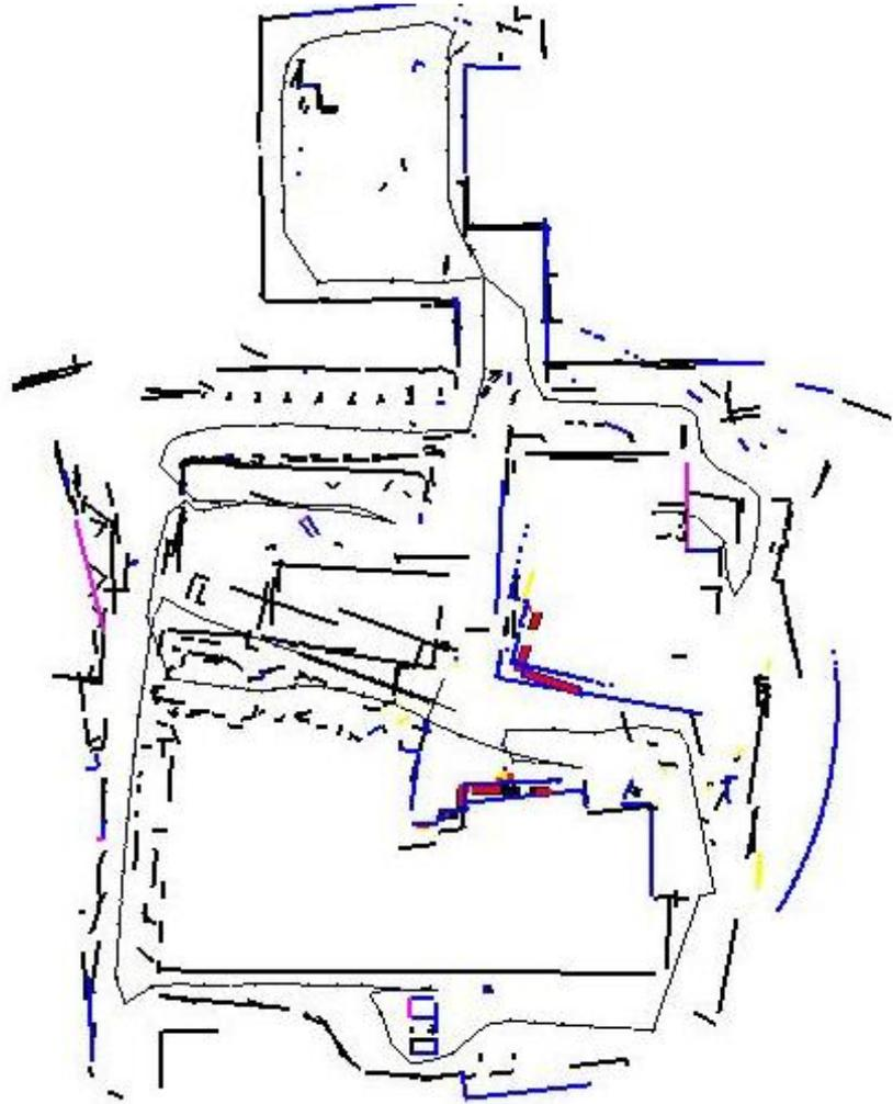
Figure 6.20: Here the robot is near the center of the map and has completed a loop around the large building in the bottom part of the figure. The loop has errors as shown by the duplication of walls.
