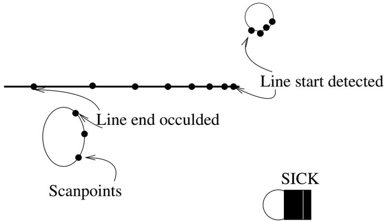
Figure 4.3: The endpoint of a line can be detected if the SICK scanner can see behind the line beyond the endpoint. Here the start of the line can be detected but not the end.
