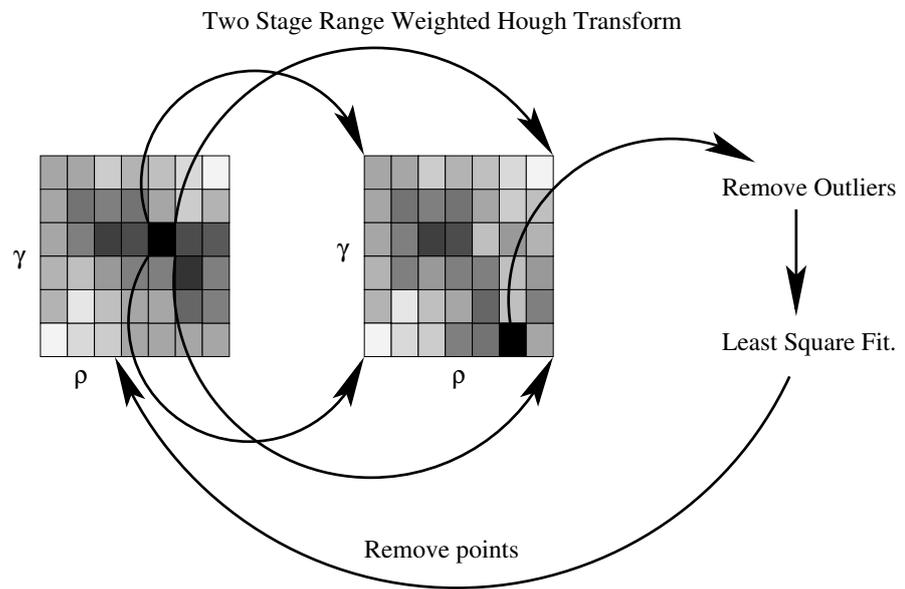
Figure C.1: The first accumulator has a coarse grid of  $\rho$  and  $\gamma$ . The maximum cell's contents is used to fill a finer grid accumulator. A preliminary fit is done to a line. After removing outlining points far off the fit line, a final fit is done adjusting the points for finite beam width. The final set of scan ranges are removed from the accumulators and a new maximum is found.
