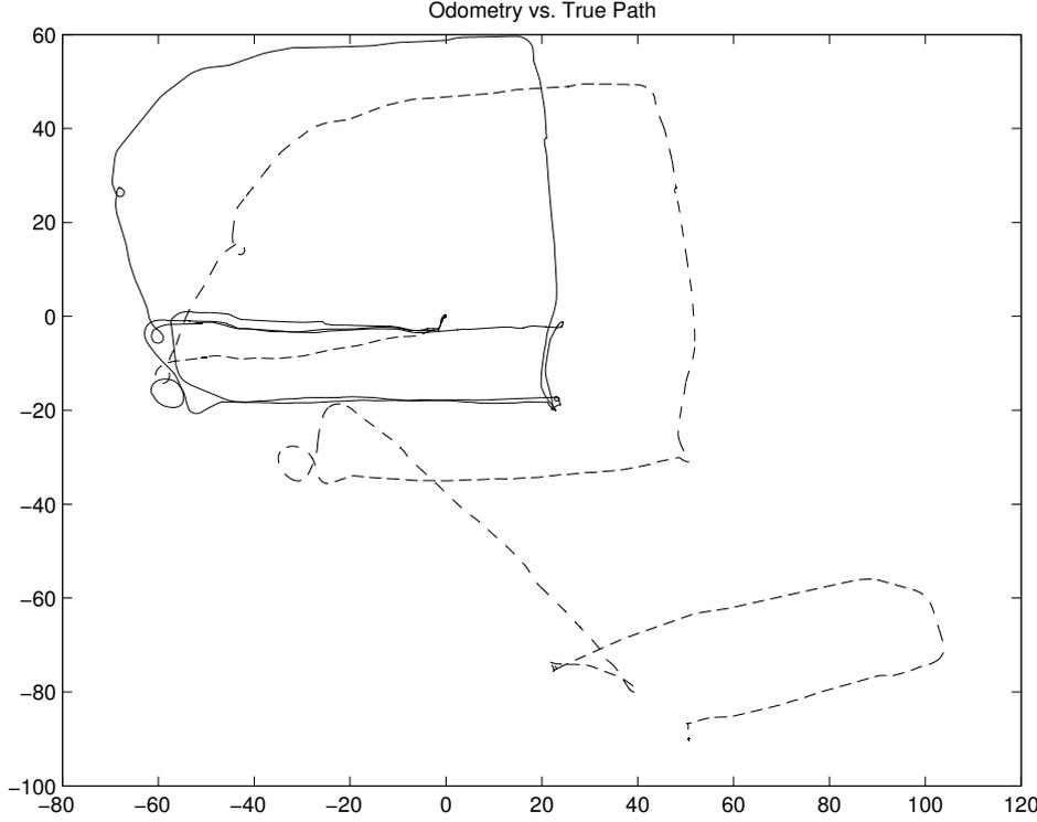
Figure 3.5: This is a typical comparison between raw odometry data (dashed) and the true path of the robot (solid). The pose error is growing without bound. The distances shown are in meters.
