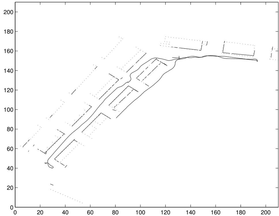
Figure 5.13: This is an example of a typical SLAM test at the mock town. The terrain behind the buildings where we start is very rough with the pitch and roll angles reaching maximums of 30, respective 10 degrees. The results show that we can build maps over the difficult terrain. The scales are in meters. The ground truth is shown as faint dotted lines for the survey map of the buildings.
