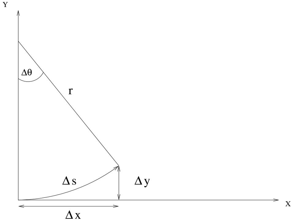
Figure 3.1: The motion of the robot over short time intervals can be approximated by motion along a circular arc.
