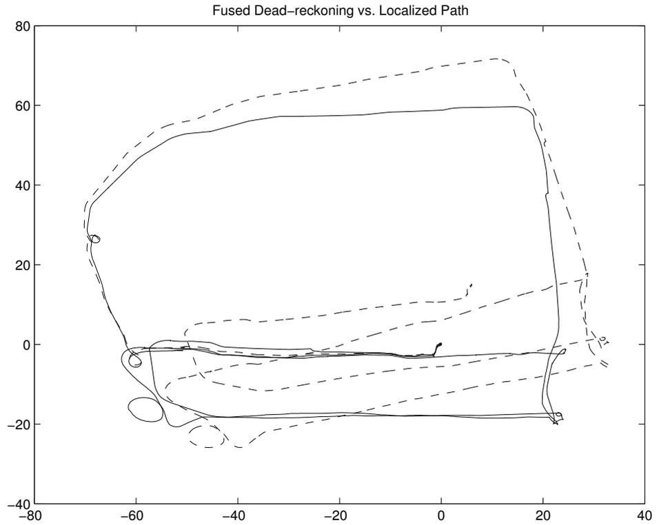
Figure 3.6: This shows how by fusing the odometry and inertial estimates (dashed line) we can get a dead-reckoning estimate far better than odometry alone. The pose error is still growing without bound. The true path is shown as the solid line. The distances are in meters.
