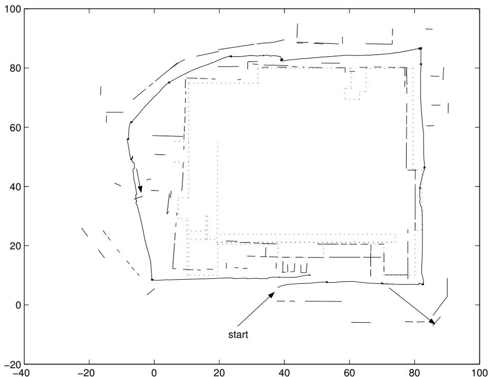
Figure 5.14: This is an example of autonomous exploration and map making. The dotted lines represent the actual building. The solid lines are the walls, fences and cars that the robot built into a map. The robot path is shown as the continuous curve encircling the building. This is also the real-time data saved at the time of the explore. Despite the errors the robot maintained a good enough pose estimate to carry out a complete exploration. Distances are in meters.
