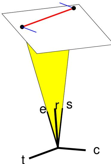
Figure 4.8: A horizontal line feature showing the 1 dimensional M-Space.
