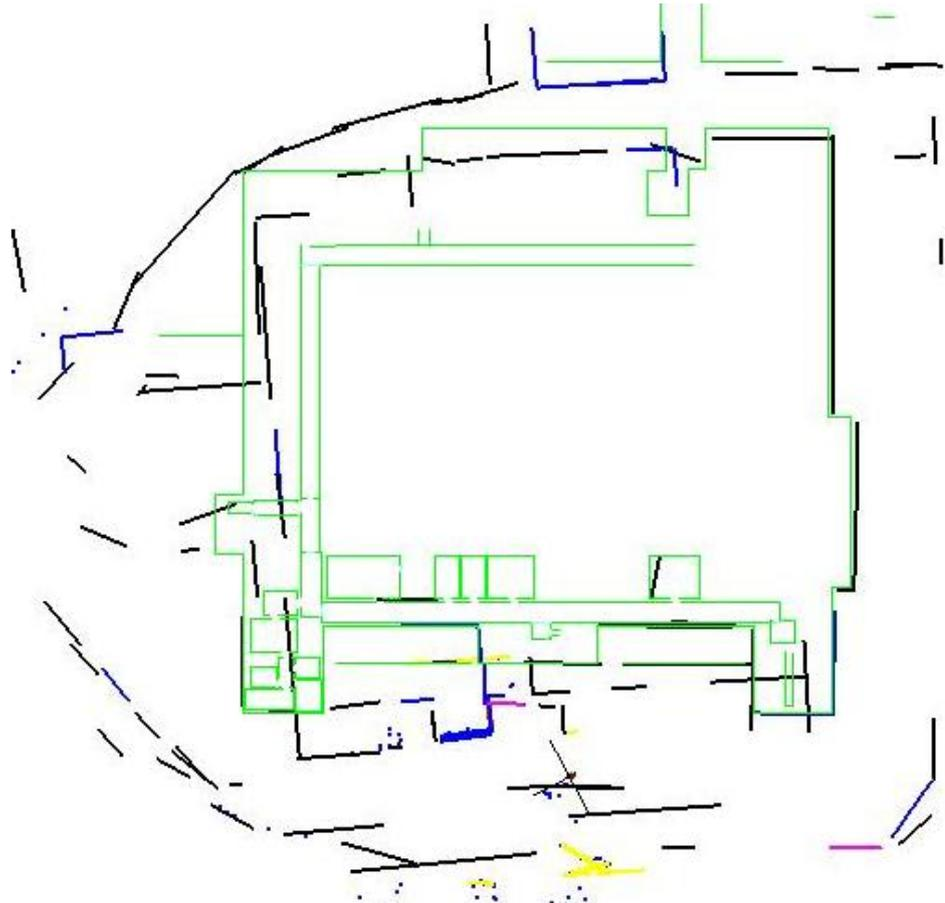
Figure 5.10: Here we show the EKF solution to a data set made with the ATRV robot exploring autonomous. The EKF algorithm cannot consistently be updated with the large error on closing the loop here. The size of this area is about 100 x 100 m.
