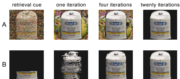
Figure 6.11. The successive retrieval of image number 9 in the COIL-100 database. The retrieval cues are shown in the left most column and the completely retrieved images in the right most column. The upper row (A) shows noise reduction from a retrieval cue with 70% noise. The lower row (B) visualizes pattern completion from a 30% partial view of the stored image.
