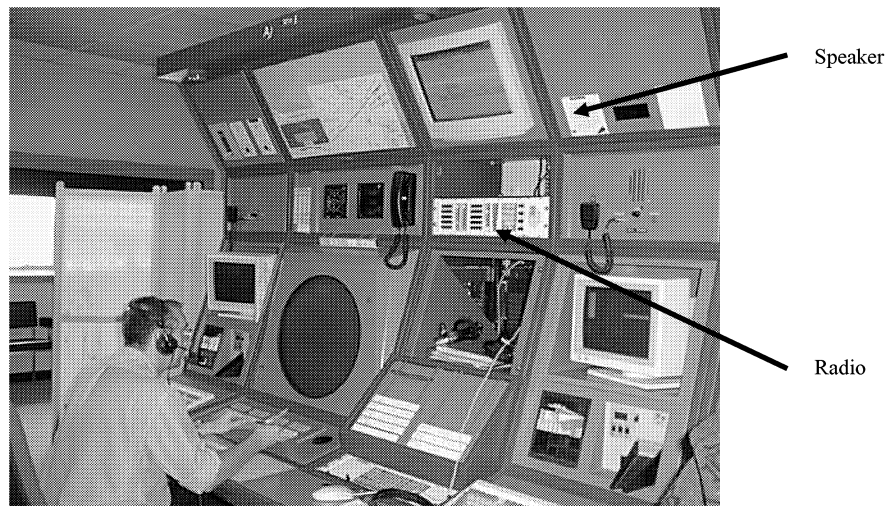
Figure 13: The approach sector with the loudspeaker that the controller uses to listen in to another sector.
