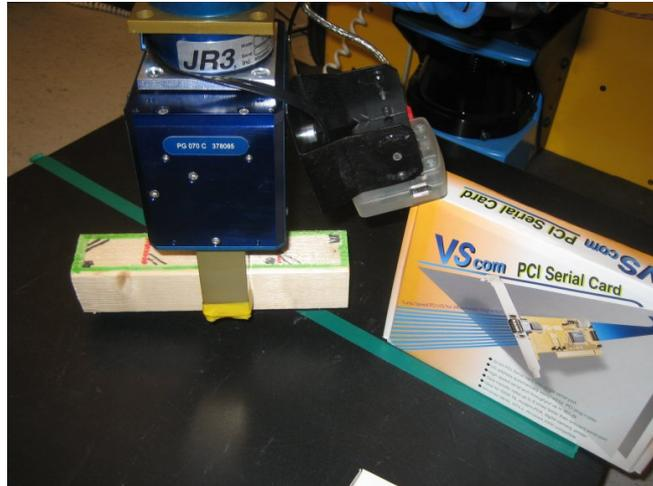
Figure 5.9: The choice of grasp type is very important. Here, the camera has not been modelled and thus the robot thinks it is fine to put down the wooden block next to the box. However, this causes a collision between the tall box and the camera.
