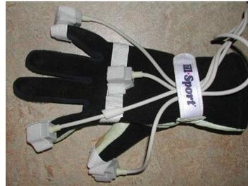
Figure 4.2: The glove used for human input.
