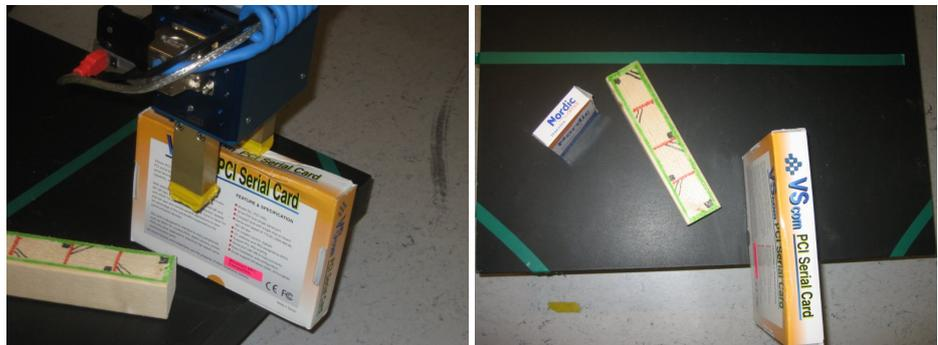
Figure 5.12: Left: The robot gripper as it about to put down the box and finish the task. Right: The final configuration of the objects, arranged by the robot. When compared with the demonstrated task, Fig. 5.11 (top-left), the configurations seem identical.
