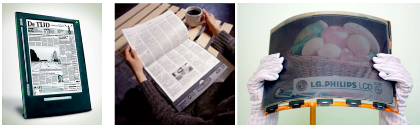
Figure 3.2 Examples of e-papers: a commercialised e-paper, and two aspiring e-papers (prototypes) (Boumans, 2006; WFU, 1999; LG.Philips, 2007).
