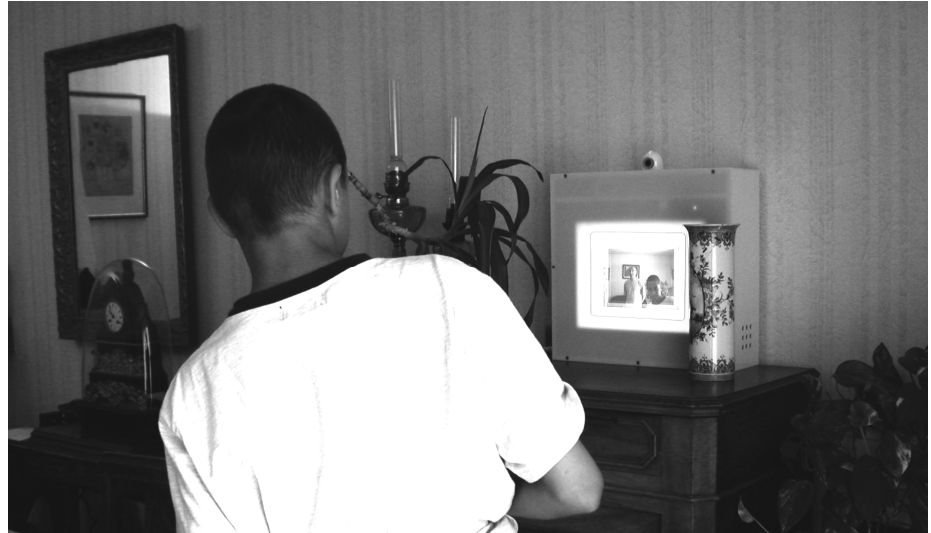
Fig. 3. The videoProbe displays still images taken at a connected remote household
