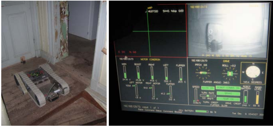
Figure 4.18. Trials were made to use the Packbot to locate IEDs. IEDs at floor level could occasionally be identified from within a few meters. The glare in the video is caused by the IR illuminator at close range.
