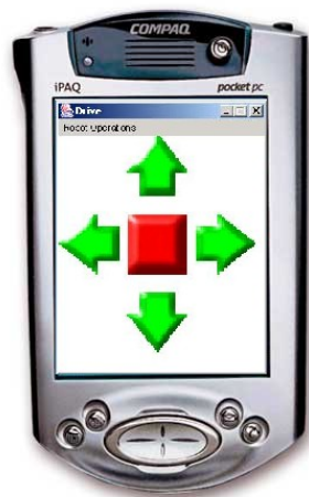
Figure 3.4. The Compaq iPAQ PDA displaying the tele-operation screen for line-of-sight tele-operation of the ATRV robot.
