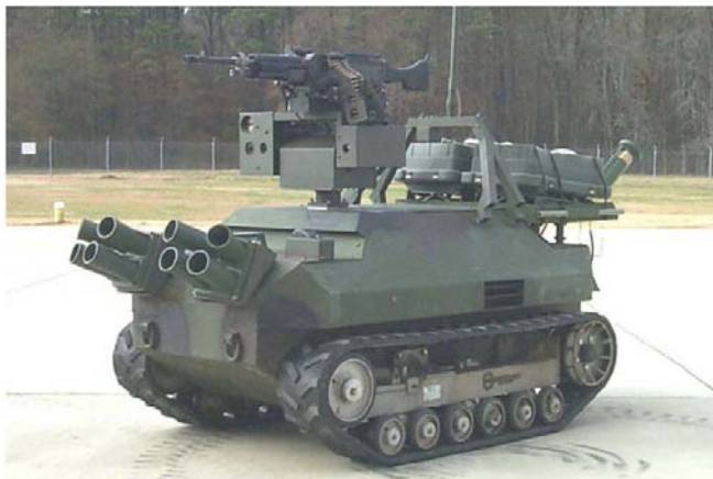
Figure 2.5. The Gladiator under development by Carnegie Mellon University in Pittsburgh for the US Marine Corps. In addition to sensors for navigation, the Gladiator is equipped with machine guns and smoke systems. It can be tele-operated up to 2-4 km.
