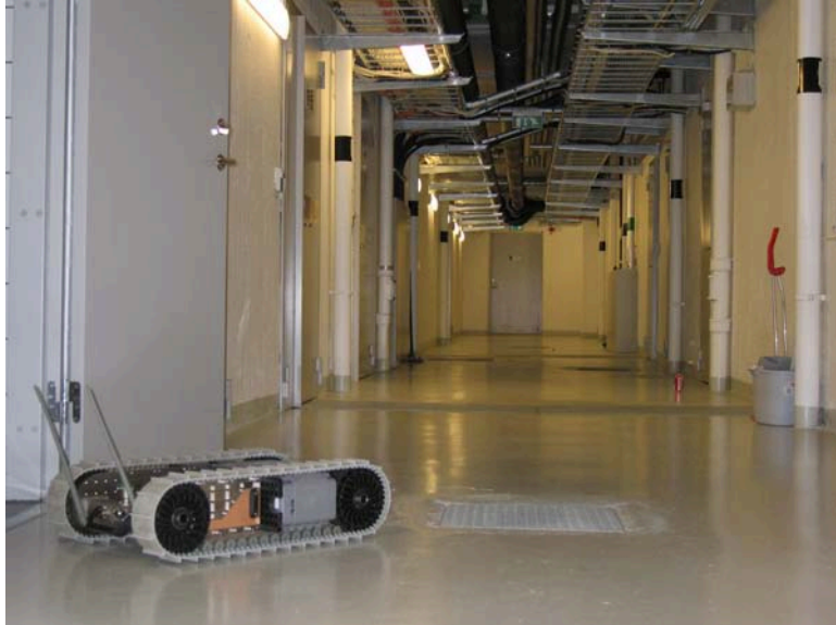
Figure 3.24. The mapping experiment was carried out in a basement and included two groups of ten test persons. One group explored the map through tele-operation and the other did the mapping by walking through the premises themselves.
