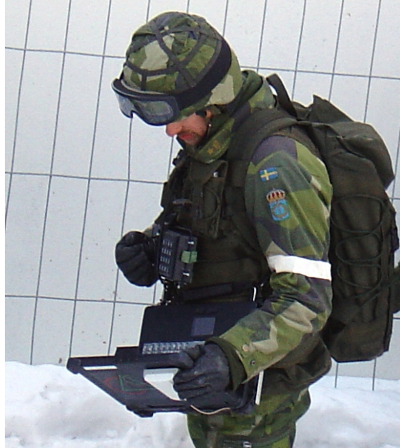
Figure 3.21. The iRobot OCU fitted with a carrying system allowing hands free portability.
