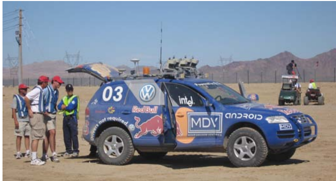
Figure 2.2. The winner of DARPA Grand Challenge 2005, the Stanford Vehicle based on a Diesel-powered Volkswagen Touareg R5 equipped with seven Pentium M computers, GPS, a 6 DOF (Degrees Of Freedom) inertial measurement unit, wheel speed encoding, laser range finders, a radar system, a stereo camera pair, and a monocular vision system.
