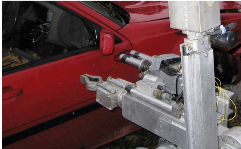
Figure 6.2. The arm of the Remotec Andros EOD robot. To the right of the gripper there are two water disruptor guns. Cable ties are taped onto the front of the disruptors to help the operator to judge the distance from the muzzle to the object. Reaching into a window of a car is a challenging task and collisions are common.
