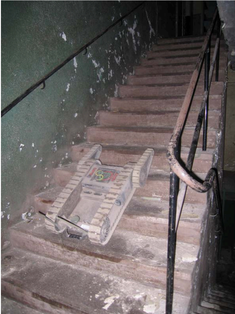
Figure 4.32. The Packbot ascending a staircase in one of the deserted steel factory in Fagersta. MOUT operations indoors are to wide extent carried out in complete darkness.
