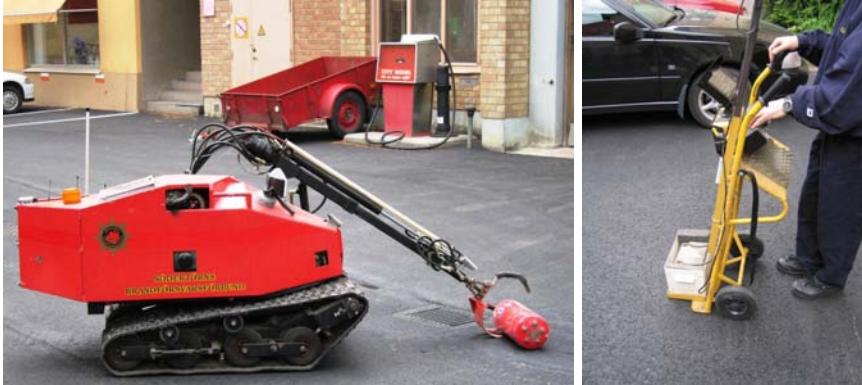
Figure 3.28. The firefighting robot – a rock-drilling machine to which has been added a gripper, three cameras and a wireless video link. The operator control unit is mounted on a sack truck.
