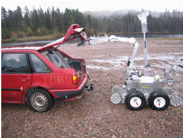
Figure 6.3. Even though it was possible to open the trunk of the car (the springs holding the hatch open were broken) the robot was unable to perform any further actions. Instead a bomb technician had to approach the site to perform the trivial task of putting a stick under the hatch to keep it open. A second, even primitive arm would be of great value on EOD missions.
