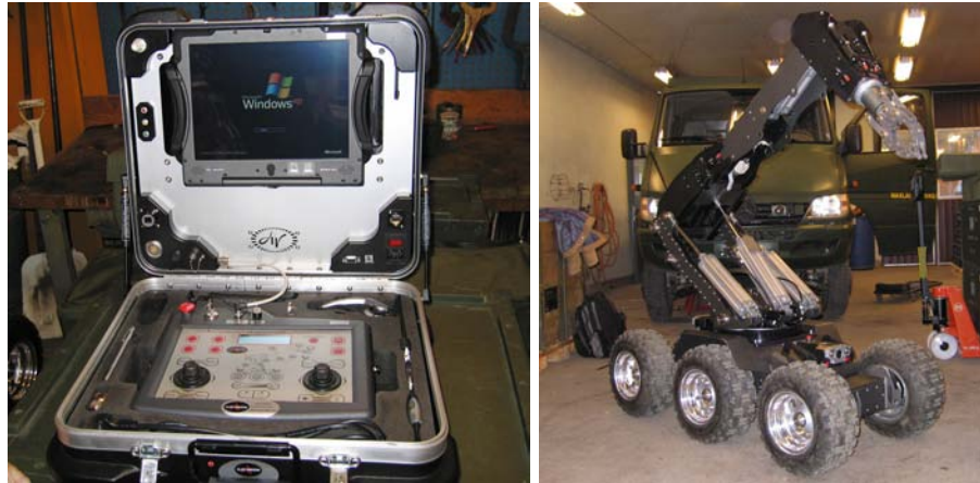
Figure 2.9. A typical field robot operator control unit (left), in this case the Allen-Vanguard Defender (right) recently acquired by the Swedish EOD units.
