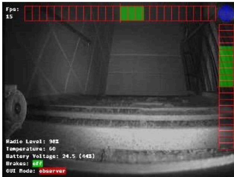
Figure 3.20. The main window of the wearable OCU showing the video with status data, speed, and turn rate overlaid.
