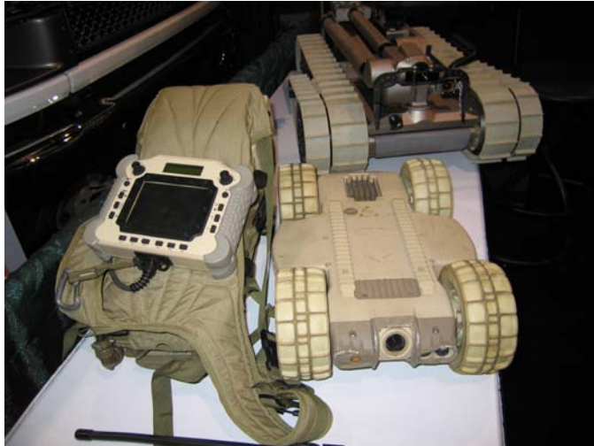
Figure 2.4. The extremely rugged Dragonrunner developed for the US Marine Corps with one of the more field-adapted user interfaces. In the background a Packbot EOD.
