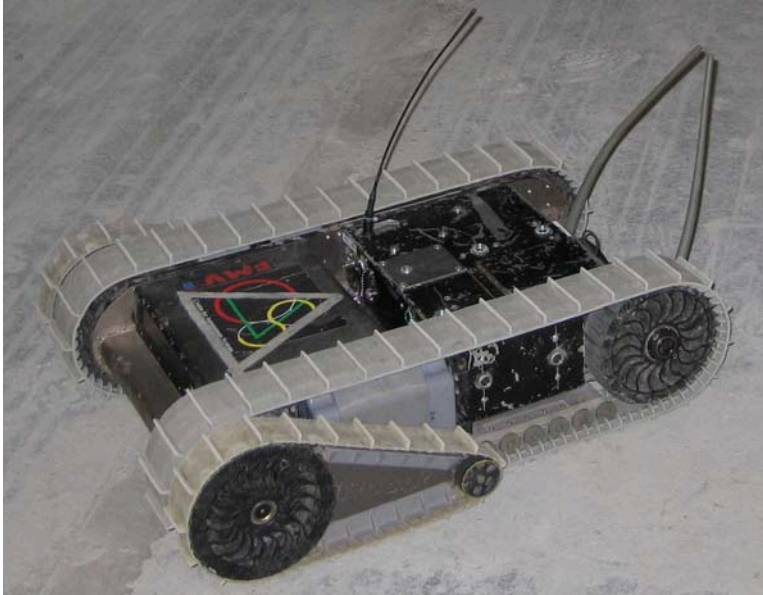
Figure 3.13. The Packbot Scout with the DFWES system enabling the soldiers to engage the robot in the same way they engage each other with firearms during training. The robot had two DFWES sensors (black circular) on each side, three on top, and two in the rear.
