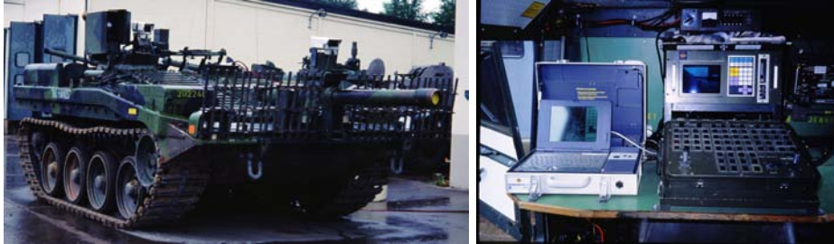
Figure 2.6. Trials to tele-operate the Swedish Main Battle Tank 103 were carried out in the early 1990s. Although all the main functions of the tank, including firing the cannon, could be executed remotely, no suitable tactical applications were identified.
