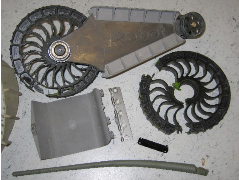
Figure 4.30. Although the Packbot is fairly sturdy it was found to have its limits. At the top a broken flipper arm, in the center holders and lid for one of the batteries and at the bottom an antenna that has come off its connector and holder after roll-over.
