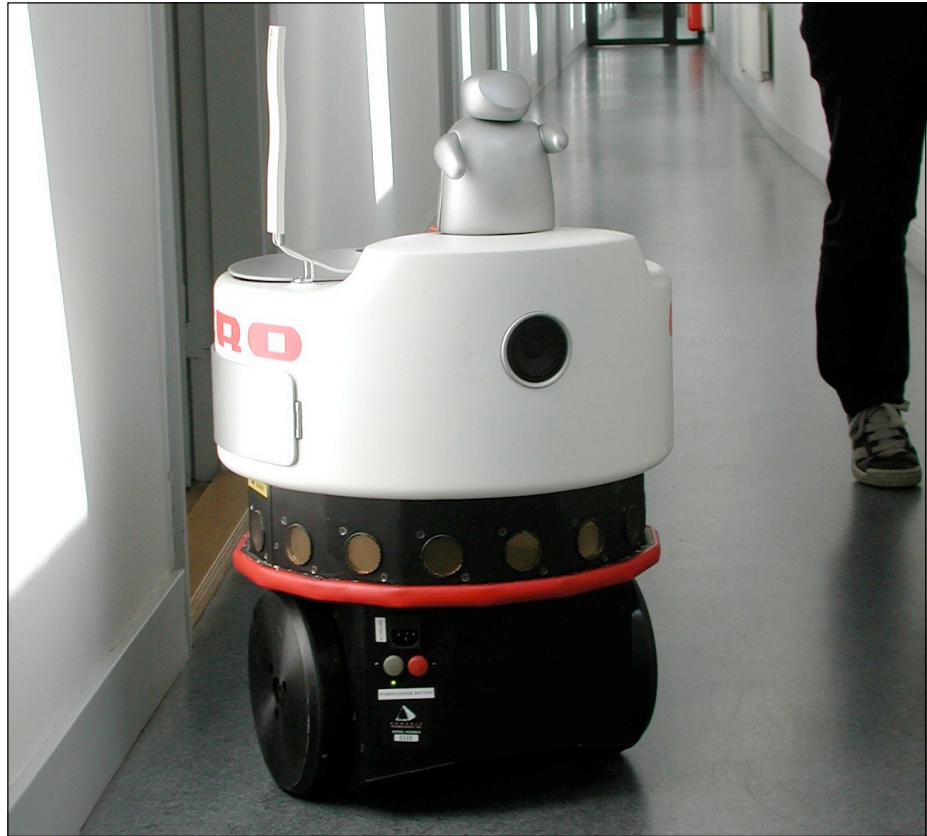
Figure 4.1 The Cero robot with its interface robot and the cover that was fitted on top of the Nomadic Scout.
