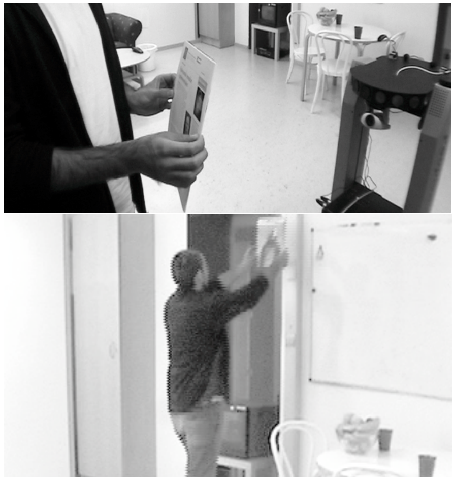
Figure 6.2 In the situation depicted in the top image, miscommunication occurs because the user is displaying an object, a magazine, in a way that the robot cannot understand (according to the constraints given by the dialogue model). In the lower image the user has adapted his behaviour to conform to the dialogue model. This is done by placing the magazine on a flat surface. In this case the user found a ledge on the wall where the magazine could be placed upright.
