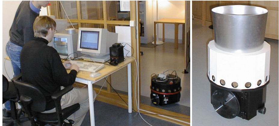
Figure 4.3 The Wizard of Oz setup (left). An early version of a casing for Cero from low-cost materials: a flower pot and cardboard that was cut and assembled to form a simple casing (right).
