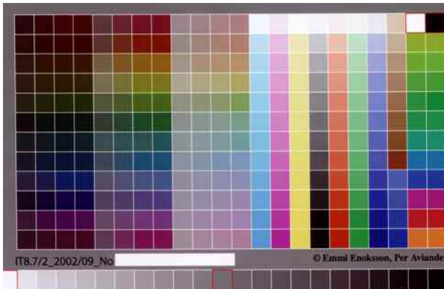
Figure 23: The customized IT8 target for scanners made by Enoksson and Aviander .
