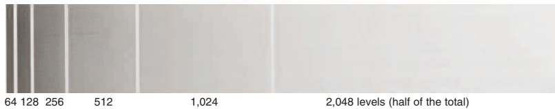
Figure 9: The six steps of dynamic range (= an analog limitation of the sensor).
