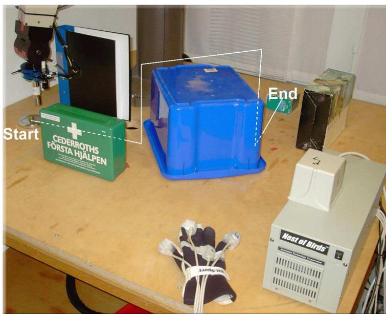
**Figure 3.8.** Typical workspace for pick-and-place task with obstacles. The white line shows the expected path of the end-effector.
