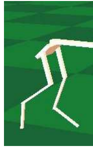
Figure 4.3: A : This figure shows a snapshot of the 3-dimensional cat model while the simulation running. Hind limbs are controlled by the muscles but the fore legs are stiff and support the trunk. Figures from B to E show screenshots of the right hind leg at different time points in the step-cycle (for clarity muscles are not shown). B : Lift off. C : Swing. D : Late swing- Touch down. E : Stance.
