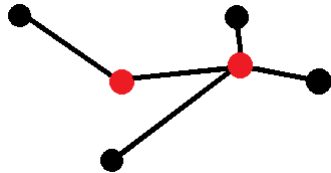
Figure 3.5: Another (sub-optimal) solution to a Steiner network problem. The solution contains two imaginary connection points colored red
