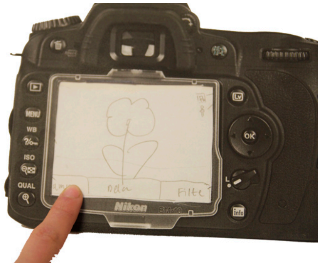
Figure 3. The prepared template of a D90 scaled 1.5 times, with a cut whole as the screen. A paper drawing of a interface made by a participant in the workshop is placed underneath the template to simulate it's screen.
