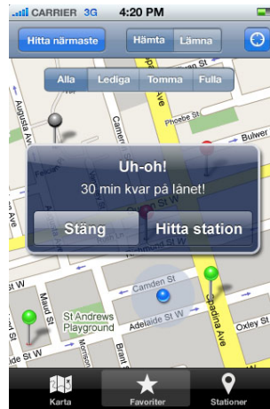
Figure 13 - Countdown timer implemented in the design.
