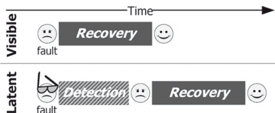
Figure 3: Types of replica faults. A sad face illustrates a fault and a happy face a successful recovery. The sad face with sunglasses illustrates a latent fault before detection. Noticeable is the difference in the time elapsed to complete recovery between the different faults.
