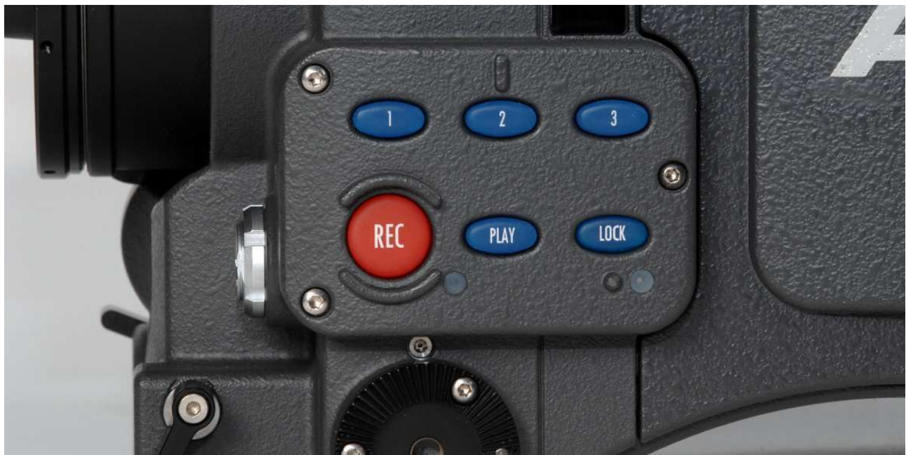
Illustration 8: User interface of the operator controls on the left side of the camera.
