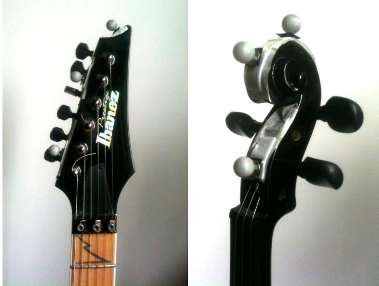
Figure 9 Guitar and violin with tracking sensors. The reflective balls define the instruments as rigid bodies.
