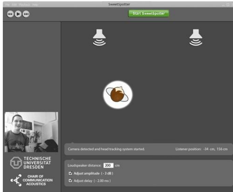
Figure 4. The Sweetspotter application where we can see the listener's position in relation to left and right speakers. The view of the camera is shown in the bottom left corner (Merchel, 2012-05.15).
