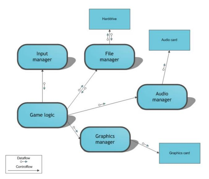
We have used a data- and control flow diagram, which shows how our system works. The rounded rectangles represents the software and the others represent the hardware. We will use the same type of diagram in following sections.
