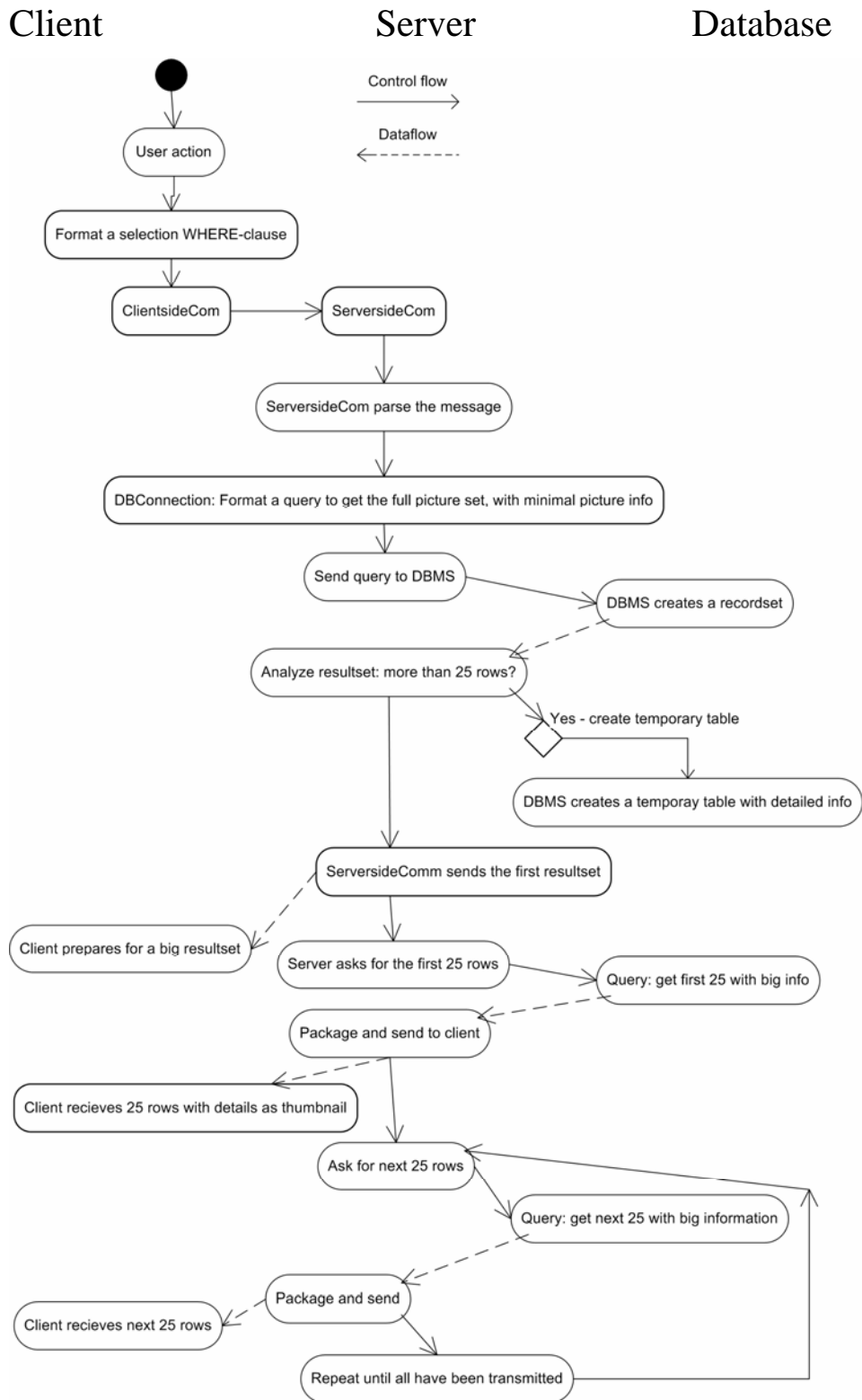
Data and control flow model (UML) for making a big (>25 rows) selection of pictures to display.
