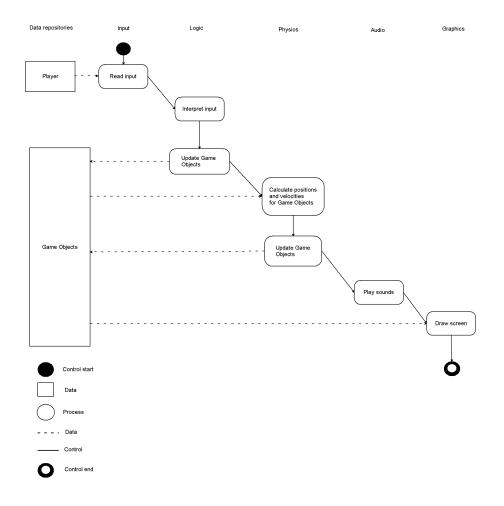
The following diagram shows data and control flow during an iteration of the game loop in the case of a player jumping.
