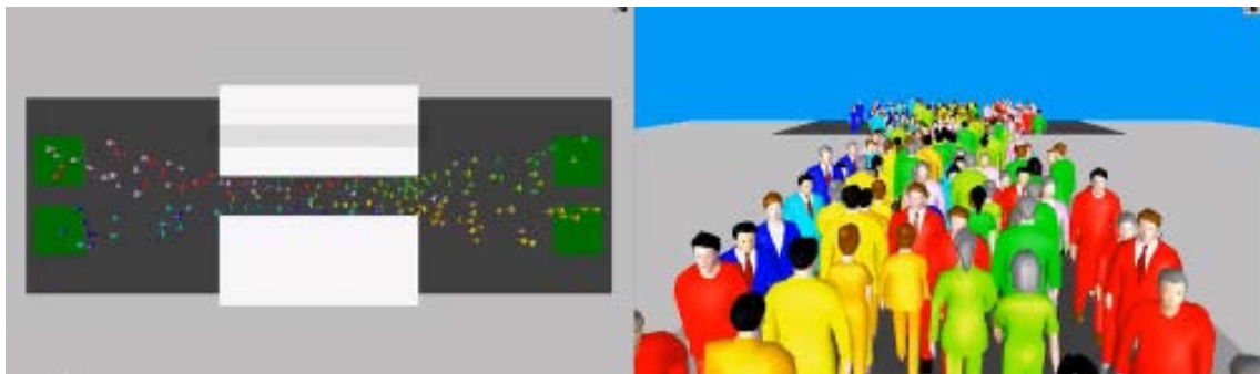
Figure 1. 2D vs 3D pedestrian simulator comparison. The crowding behavior looks realistic in the top-down 2D view but in the 3D view one can see pedestrians that are lining up against the wall and bumping into each other.
