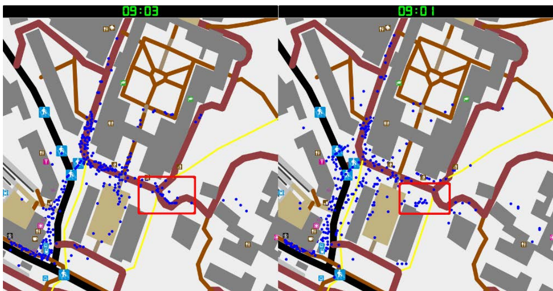
Figure 7. On the left side a lower weight for the heuristic is used – resulting in pedestrians who follow the footway. On the right side a higher weight is used, improving the performance slightly, but with pedestrians that do not follow the footways.
