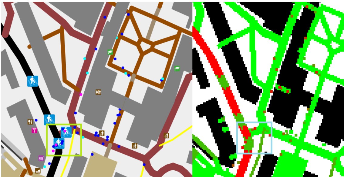
Figure 5. Example of pedestrians using a crossing. The snapshot to the right shows the cost matrix where black indicates unwalkable areas, red indicates areas with a high cost i.e. should be avoided if possible, green indicates areas with a low cost and white indicates neutral areas that have medium cost.
