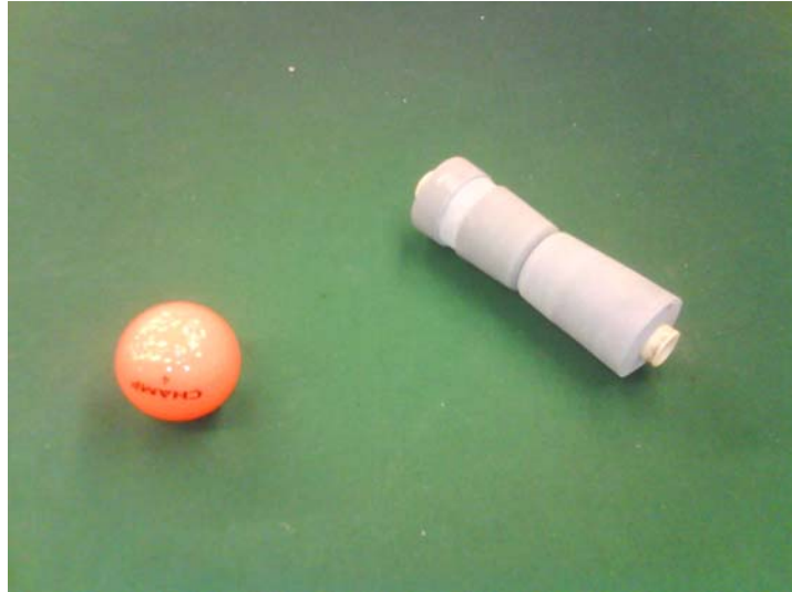
The two door stoppers mounted on PVC tubing
