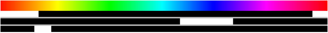
Each object has a defined hue interval shown in the picture. From top to bottom; ball, blue goal, yellow goal (without edge detection algorithm).
