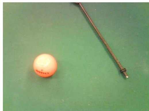
Vulcanized tape on steel rod. High grip, symmetrical. Too hard.
