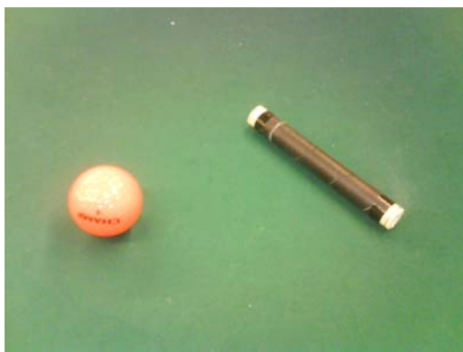
Tennis racket hand grip tape. Good grip, unsymmetrical, vibrating. Too hard.
