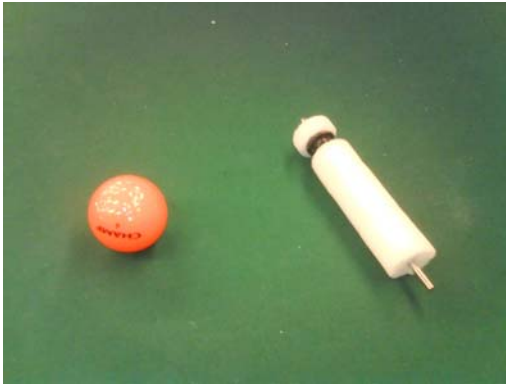
Soft foam on steel rod. Good grip, unsymmetrical, too soft.
