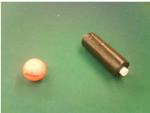
Vulcanized tape coating on foam cylinder mounted on PVC tubing. Good grip, unsymmetrical, vibrating.
