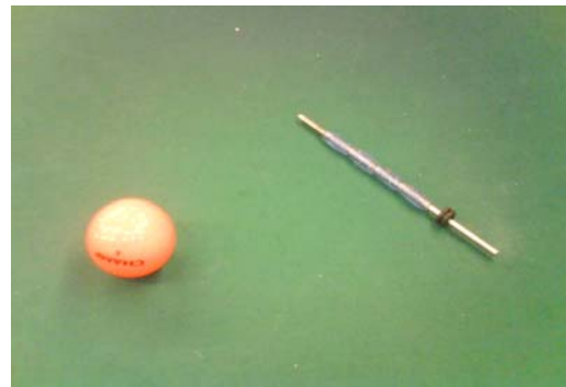
Small fishing jigs threaded on steel rod. Very high grip, no vibration, unsymmetrical.
