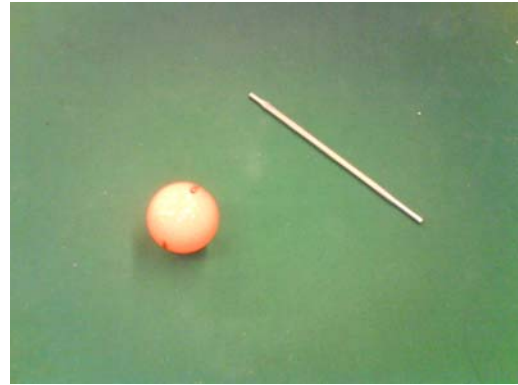
Smelted glue on steel rod. Good grip, symmetrical, no vibration. This was a good candidate, but it was too hard.
