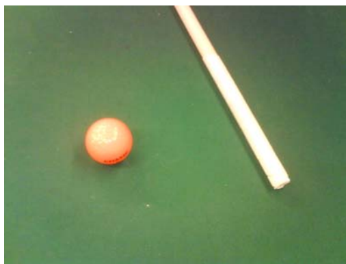
Double sided tape on PVC tubing. Due to rule violation where the ball would get stuck permanently on this roller, it was not tested further.
