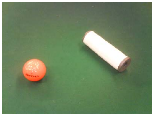
Electric tape on foam cylinder. No grip, unsymmetrical vibrating.
