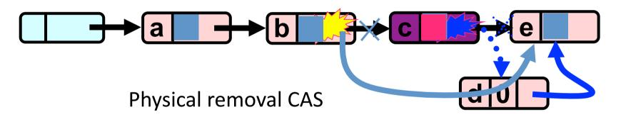
Mark-Bit and Pointer are CASed together (AtomicMarkableReference)
