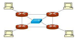
Connect fe-2/0/0 to the hub at the bottom of your rack to study OSPF over a transit network with more than two routers. Use the addresses assigned in the topology map.
