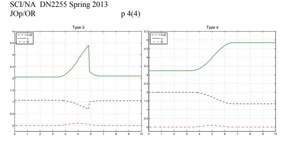
*Note the small entropy-violating "shocklet" in type 3... the entropy fix should be strengthened.*
