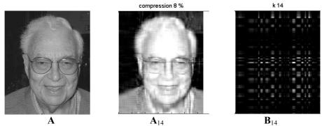
The rank-1 character of  $\Delta A_{14}$  is revealed by its obvious row and column structure. The approximation error is in short wavelength features, it looks much better after blurring a little. This is easy to show with a projected image by turning the lens slightly out of focus ... unless the projector has auto-focus like the one used in the class. I suspect that JPEG (lossy) compression does better than this.
