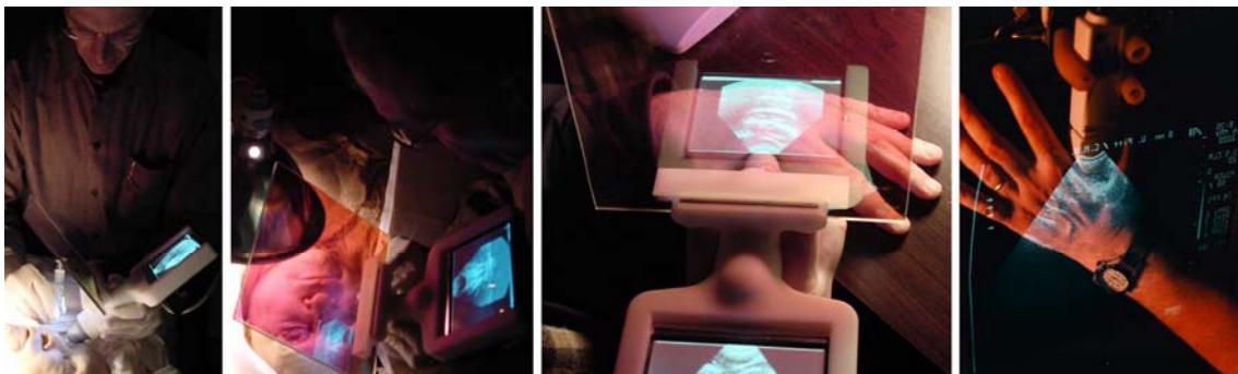
Figure 1. The Sonic Flashlight uses a see-through display to overlay real-time ultrasound images over a patient's body parts. (Images courtesy of George Stetten [Stetten et al. 2001].)
