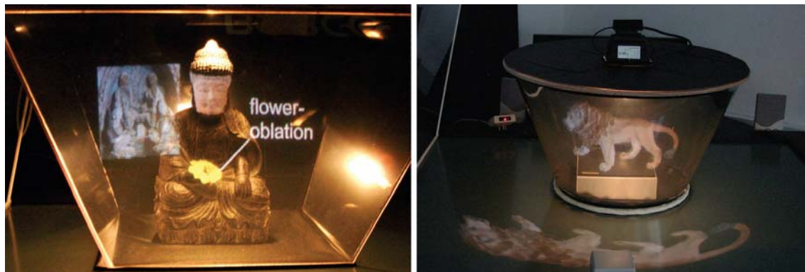
Figure 4. The Virtual Showcase augments physical objects inside showcases with dynamic annotations or related media. The Virtual Showcase is covered with half-silvered mirrors that optically combine the view of the objects with computer graphics reflected from the rear-projected table, on which the showcase is placed. (Images courtesy of Oliver Bimber [Bimber et al. 2003, Bimber et al. 2001].)
