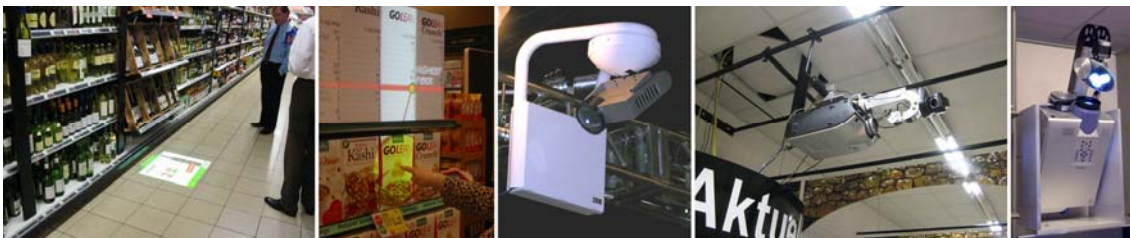
Figure 9. The Everywhere Displays project uses “steerable displays”, where the system’s projector can create augmentations on different surfaces in the environment, while the camera senses the user’s interaction. (Images courtesy of Claudio Pinhanez [Pinhanez et al. 2003, Pinhanez and Pingali 2004, Pinhanez and Podlaseck 2005, Pinhanez 2001].)
