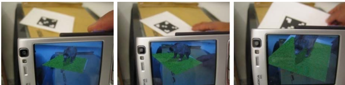
Figure 7. Video see-through AR can be achieved using commercial camera phones. The camera on the back of the device captures video of the real environment, which is used by software on the device to recover the phone’s pose relative to tracked features in the environment. This makes it possible to render 3D objects that are registered with the real environment, overlaid on the video that is shown on the phone’s display [Henrysson 2007].
