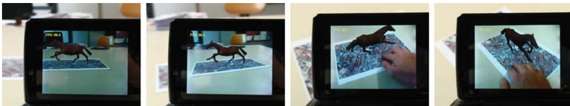
Figure 11. Natural feature tracking techniques make video see-through AR possible without the need for fiducial markers in the environment. Here, a mobile device tracks features on a printed page and overlays registered 3D graphics at interactive frame rates. (Images courtesy of Daniel Wagner and Graz University of Technology [Wagner et al. 2008b].)
