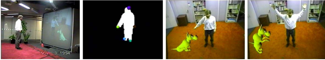
Figure 14. The ALIVE system tracks a user’s body parts and supports full body interaction with virtual creatures. (Images courtesy of Alex Pentland, Bruce Blumberg and Trevor Darrell [Maes et al. 1995].)
