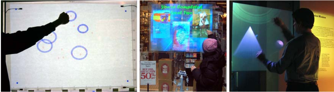
Figure 12. An acoustic tap tracker allows touch-screen interaction in public spaces by sensing the position of knocking actions on glass surfaces. (Images courtesy of Joseph Paradiso [Paradiso 2003, Paradiso et al. 2000].)
