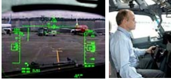
Boeing Next-Generation 737 (2003) visibility min w/o HUD: 182 m visibility min with HUD: 91 m
