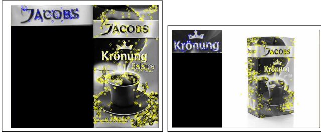
Fig. 4. Detection of objects by partial textures. Left part shows that only a “Jacobs” sign is sufficient, while the right part implies the same for a “Kronung” sign.
