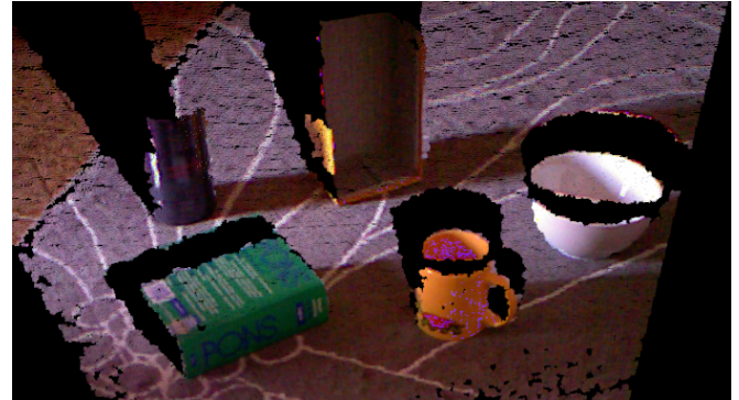
Fig. 3. Top: A scene recognized with CVFH. The CAD models are overlapped on the scene together with the 0-order affordances that each object provides. Hidden affordances are shown in red and usable affordances are shown in green. The green points represent the matching training view and the red points the points coming from the depth sensor. Best viewed in color. Bottom: Same scene from the Microsoft Kinect with color image overlayed. Note the difference between the CAD models used to trained CVFH and the data obtained from the Kinect. The recognition of the shoe box shows an example of how CVFH can deal with occlusions.
