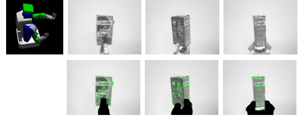
Fig. 5. Top row: Robot (left-most image) is manipulating an object in front of the camera Bottom Row: Extraction of keypoints and masking of robot's parts.
