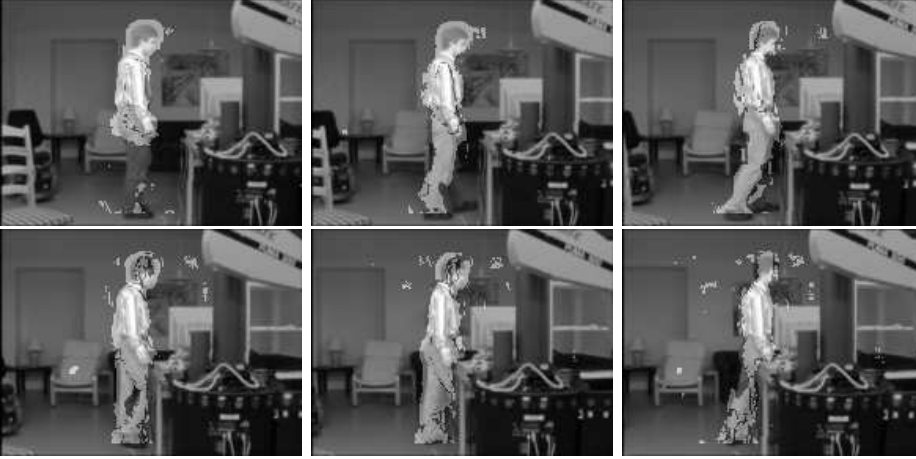
Figure 8.2. Pixels for which the probability of an object of interest is greater than 50%, based on prior distributions of disparity and optical flow.
