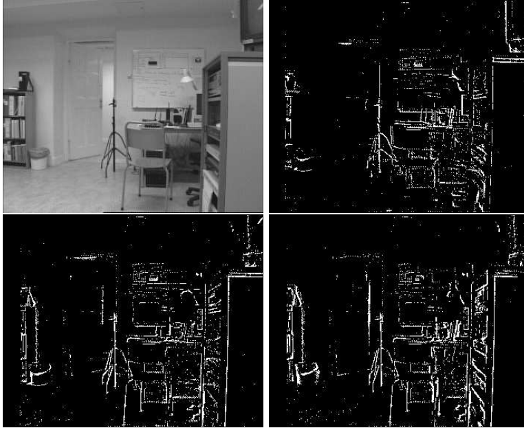
Figure 3.8. An image extracted while letting a camera pan from right to left (upper-left) and images showing points with errors in pixel value more than 8 after stabilization, for methods using corner features (upper-right), contour points (lower-left) and image gradients (lower-right).
