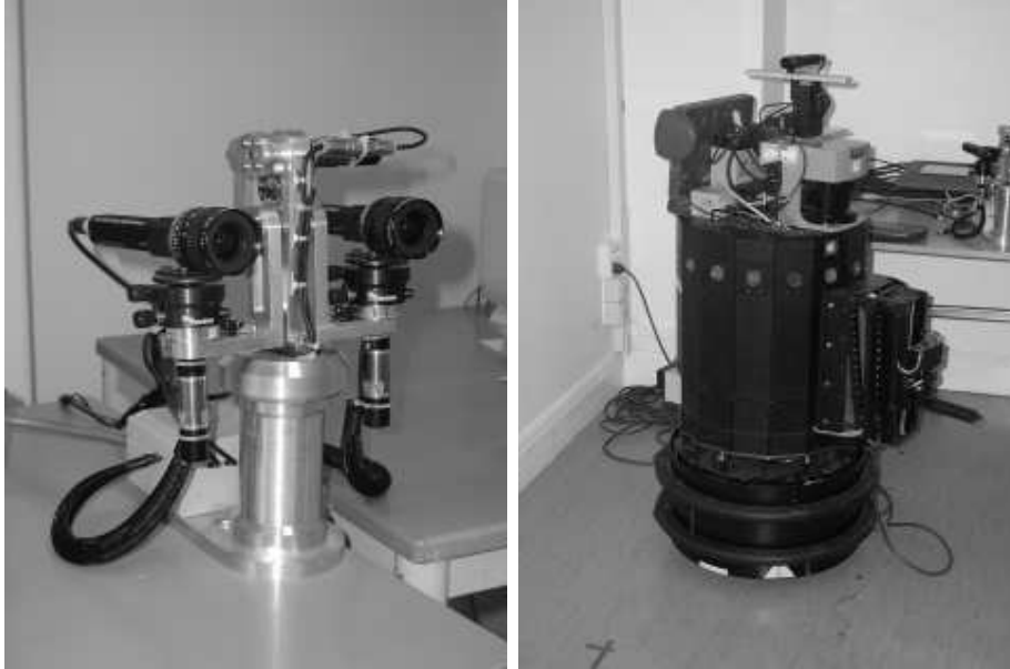
Figure 1.1. A Yorick stereo head (left) and a Nomad 200 platform (right).
