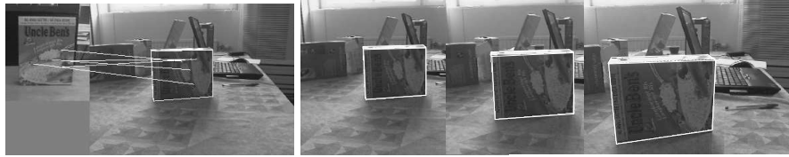
Fig. 4. Left) Initializing pose tracking using SIFT features, Right) Pose tracking.
