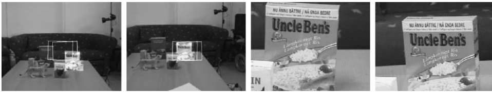
Fig. 5. The first two images show a target region before and after a saccade (the rectangles show the foveal regions within the left peripheral camera image) and the foveal camera images after executing a saccade are shown in the last two images.
