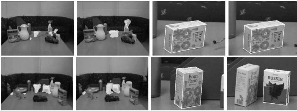
Fig. 11. The imperfect segmentation does not effect the final pose estimate of the object. The examples show when: (upper) Only a fraction of the object was segmented, and (lower) Two hypotheses are overlapping.
