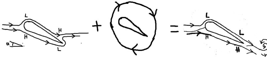
Figure 1: Potential flow (left) past a wing section with zero lift/drag modified by circulation around the section (middle) to give Kutta-Zhukovsky flow (right) leaving the trailing edge smoothly with downwash/lift and a starting vortex behind, but without viscous drag.
