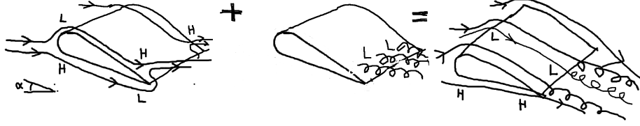
Figure 6: Stable physical 3d turbulent flow (right) with lift/drag, generated from potential flow (left) by a perturbation at separation consisting of counter-rotating rolls of streamwise vorticity (middle), which changes the pressure at the trailing edge generating downwash/lift and drag.
