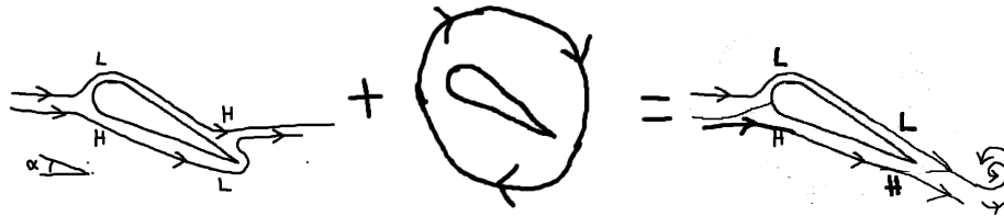
Figure 5: Potential flow (left) past a wing section with zero lift/drag modified by circulation around the section (middle) to give Kutta-Zhukovsky flow (right) leaving the trailing edge smoothly with downwash/lift and a starting vortex behind, but without viscous drag.
