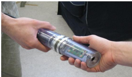
Fig. 3. The object Bidule can measure the interaction forces that occur during the object exchange.
