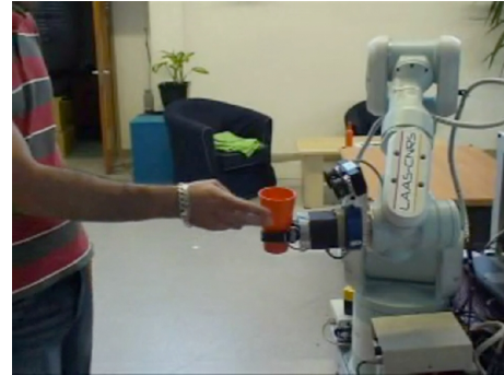
Fig. 4. This picture shows a human just touching the object; the detector does not misinterpretes this as a grasp and the grip does not open.
