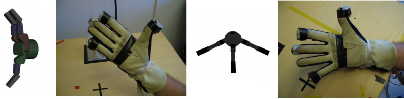
Figure 5.6: First alternative training postures to control all DOF of a Barrett hand. The distance between the index and little finger is used to control the spread angle.
