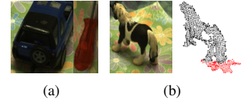
Fig. 6. Examples of imperfect segmentation in both 2D and 3D: (a) only a part of an object is detected, or (b) the segmentation mask contains background points (background points are marked in red).
